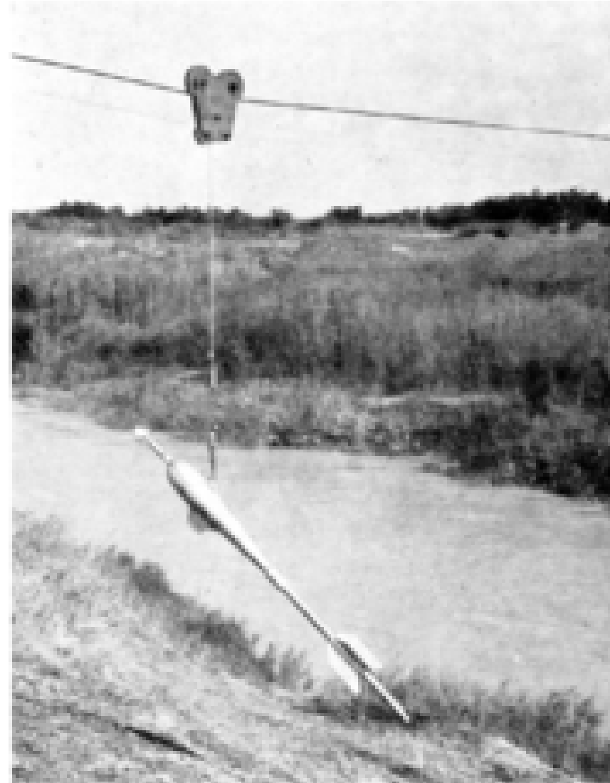
Fig. 4.12(b) Neyrtec Type Meter in a Cableway
