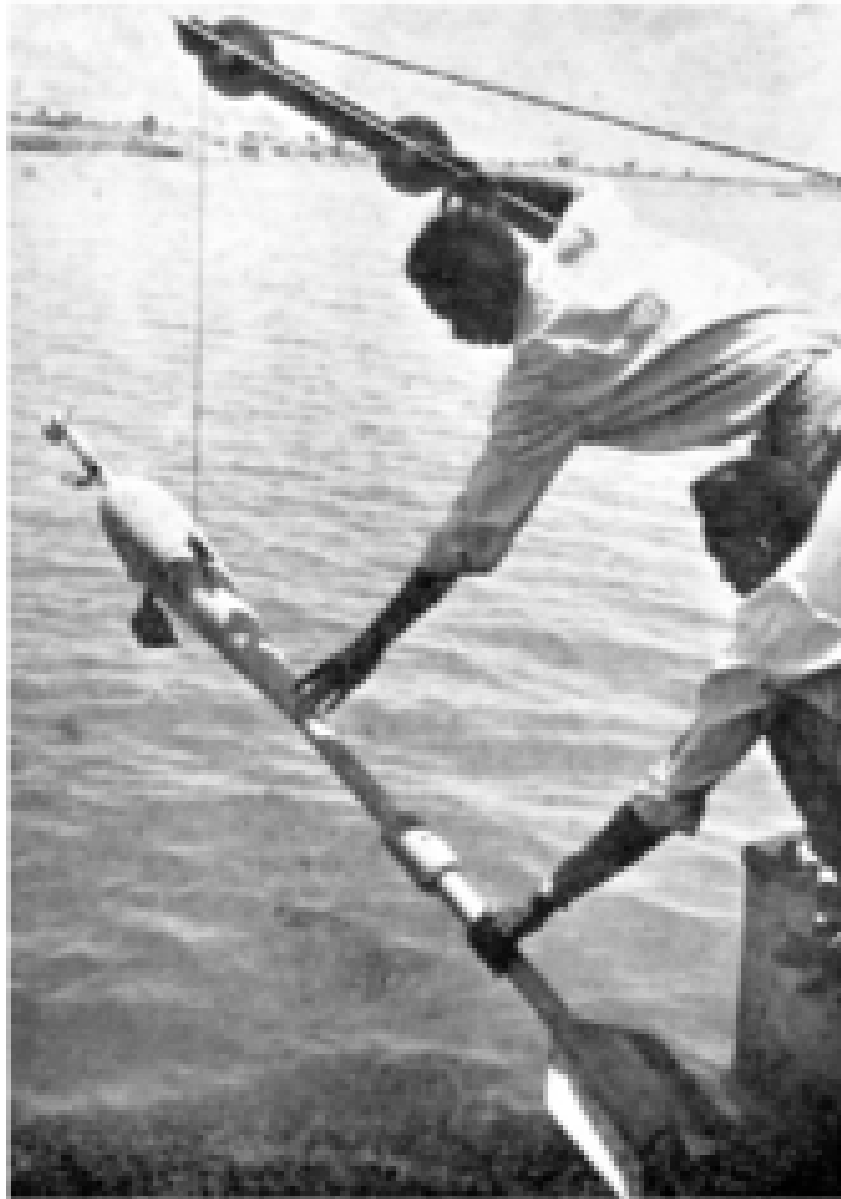
Fig. 4.10 Propeller-type Current Meter—Neyrtec Type with Sounding Weight
