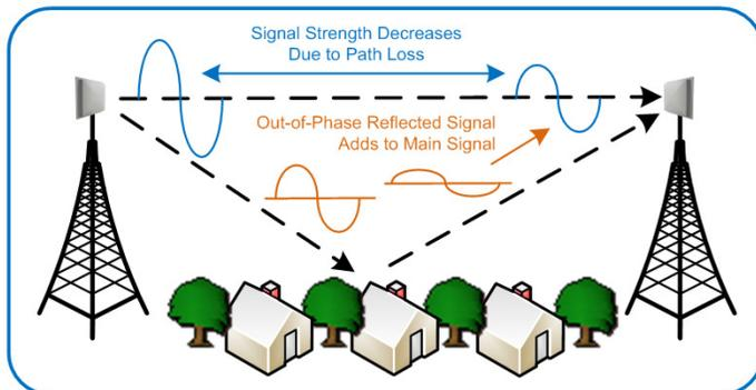
The amount of extra RF power radiated to overcome this phenomenon is also referred to as fade margin. The exact amount of fade margin required depends on the desired reliability of the link, but a good rule-of-thumb is to maintain 20dB to 30dB of fade margin at all times.
