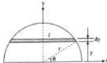
**Figure 8.8** Centroid calculation of a semicircular disk using a horizontal strip
