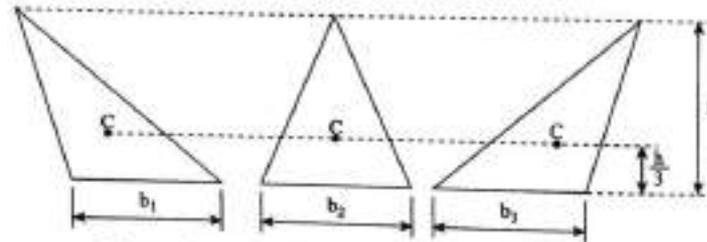
Figure 8.7 Centroid of triangles with the same altitude
