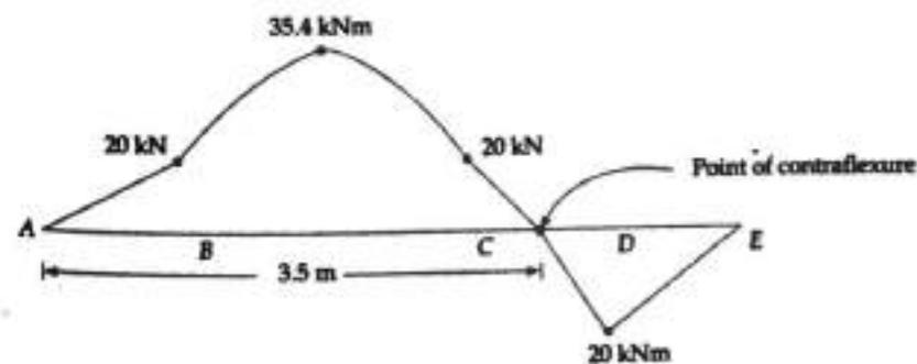
9. Determine the reactions and construct the shear force and bending moment diagrams for the simply supported beam loaded as shown in Fig. 11.51. Also determine the position and magnitude of maximum bending moment.
