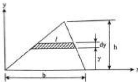
Figure 8.6 Centroid calculation of a triangle
