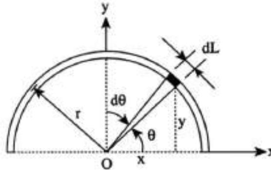
**Figure 8.1** Centroid calculation of a semicircular arc
