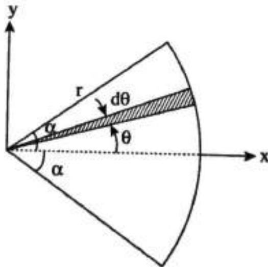
**Figure 8.13** Centroid calculation of a circular sector
