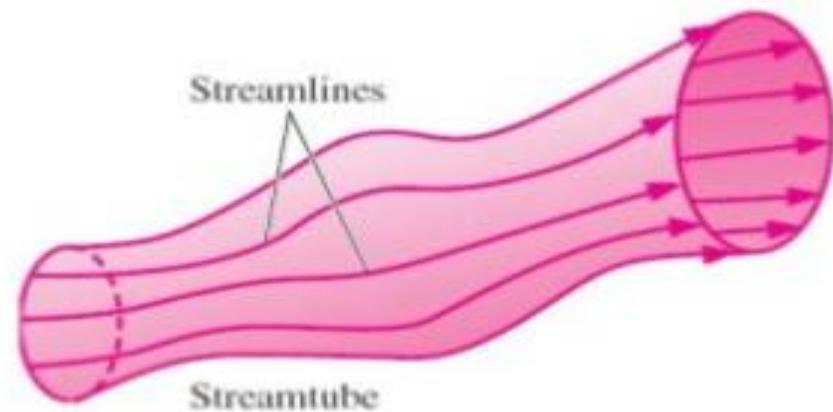
Both streamlines and stream tubes are instantaneous quantities, defined at a particular instant in time according to the velocity field at that instant.
