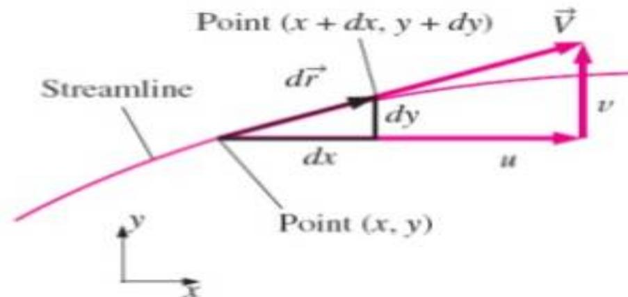
For two-dimensional flow in the  $xy$ -plane, arc length  $d\vec{r} = (dx, dy)$  along a *streamline* is everywhere tangent to the local instantaneous velocity vector  $\vec{V} = (u, v)$ .
