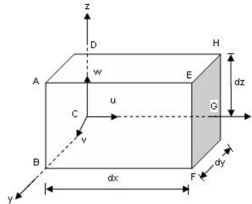
Mass of fluid entering the face ABCD per second = Density x velocity in x direction x Area ABCD
