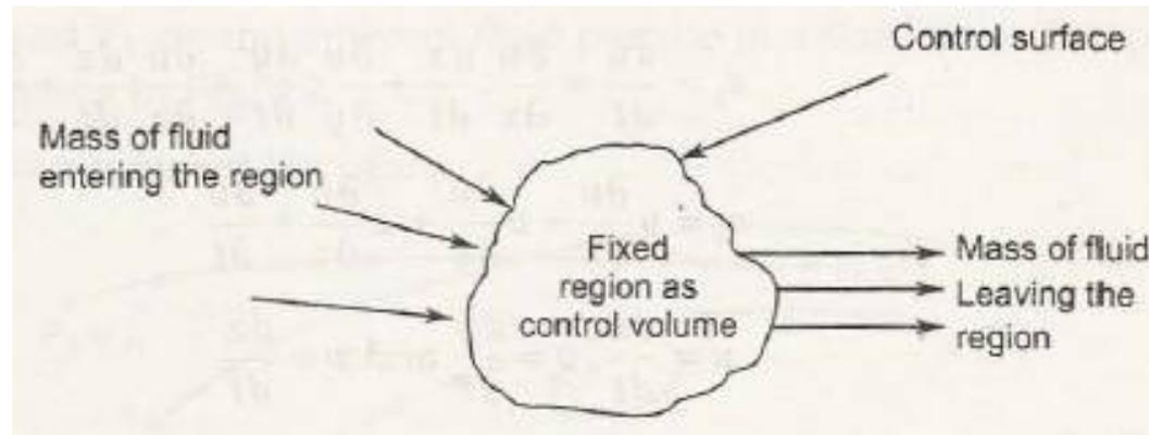
Above fig explains the concept of control volume and control surface.
