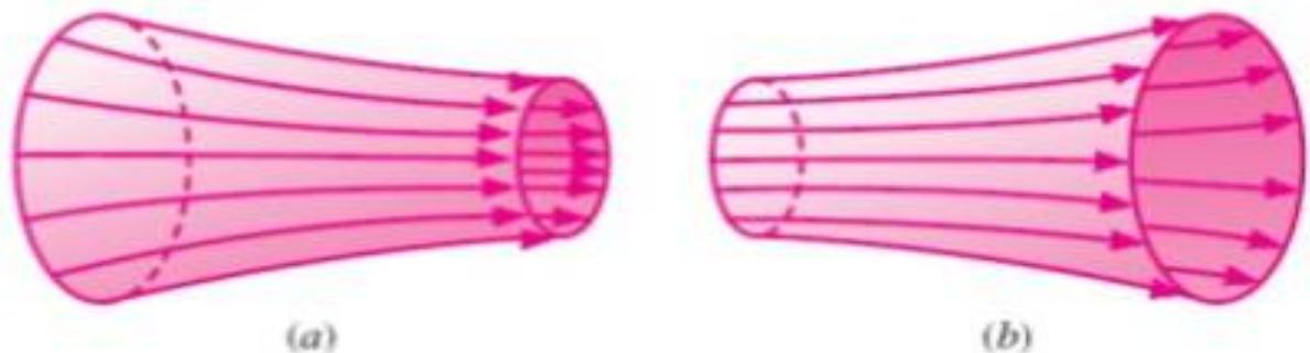
In an incompressible flow field, a stream tube (a) decreases in diameter as the flow accelerates or converges and (b) increases in diameter as the flow decelerates or diverges.
