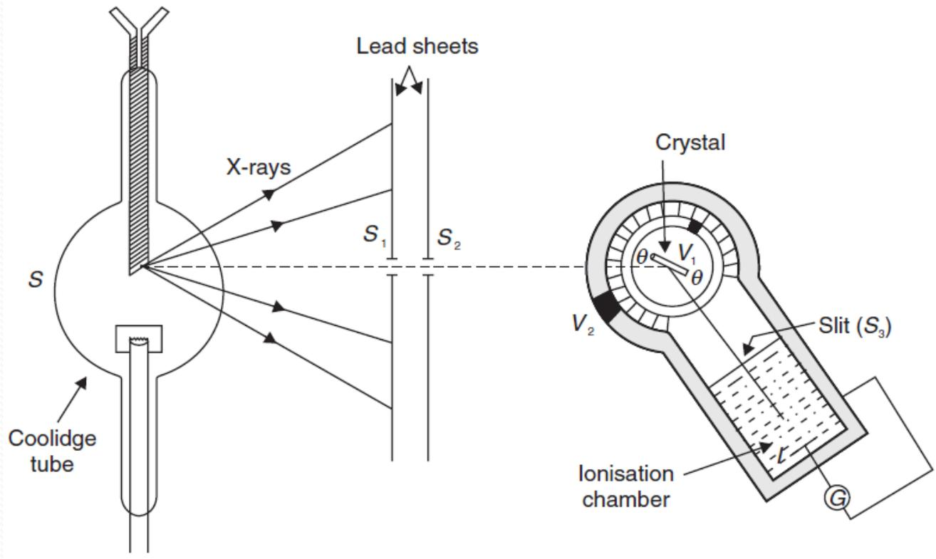
**Fig. 4 Bragg's spectrometer**
