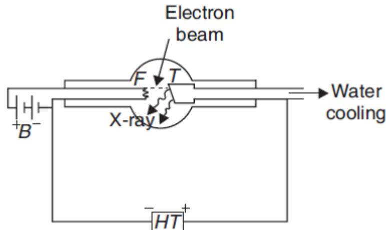
**Fig 1: Coolidge tube producing X-rays**
