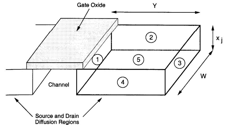
**Figure 3.33** Three-dimensional view of the n<sup>+</sup> diffusion region within the p-type substrate.
