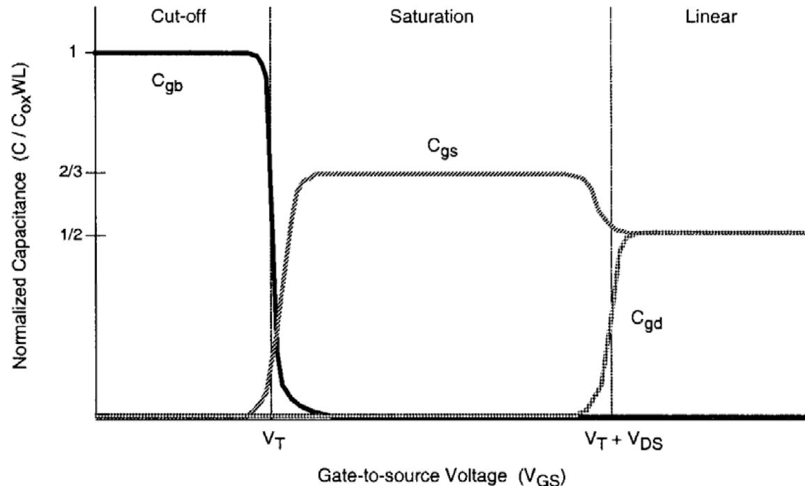
**Figure 3.32** Variation of the distributed (gate-to-channel) oxide capacitor functions of gate-to-source voltage  $V_{GS}$ .
