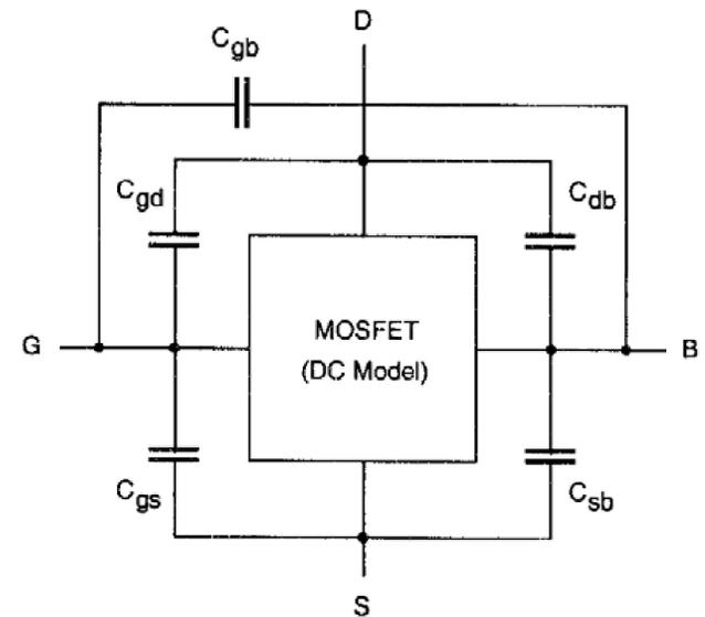
**Figure 3.30** Lumped representation of the parasitic MOSFET capacitances.
