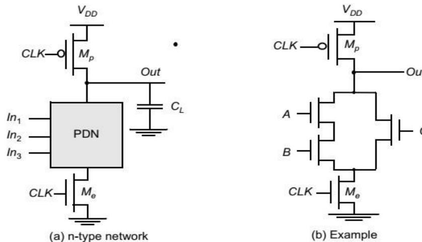
Fig. Basic concepts of a dynamic gate.
