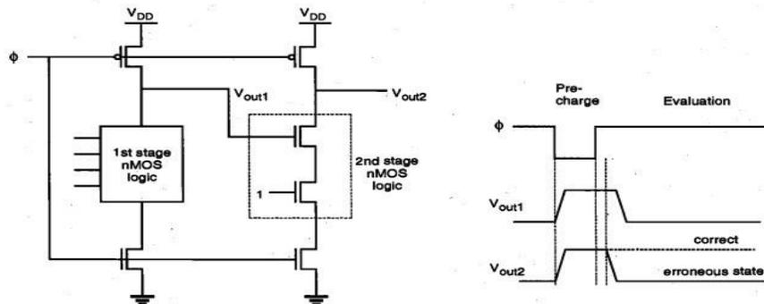
**Fig.** Illustration of the cascading problem in dynamic CMOS logic.
