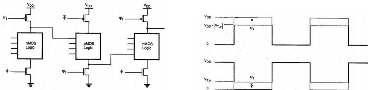
**Fig.** General circuit structure and the clock signals of Zipper CMOS
