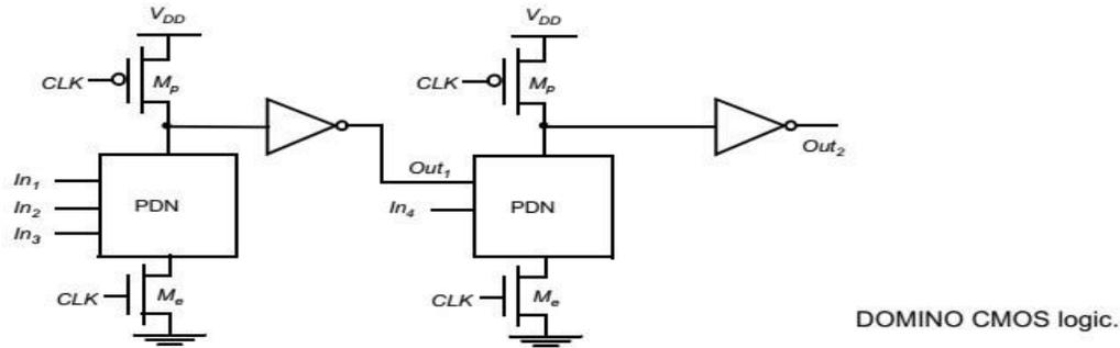
Remember that the problem in cascading conventional dynamic CMOS stages occurs when one or more inputs of a stage make a 1 to 0 transition during the evaluation phase, as illustrated in Fig below.
