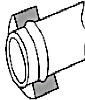
Tube is expanded into die to form beading
