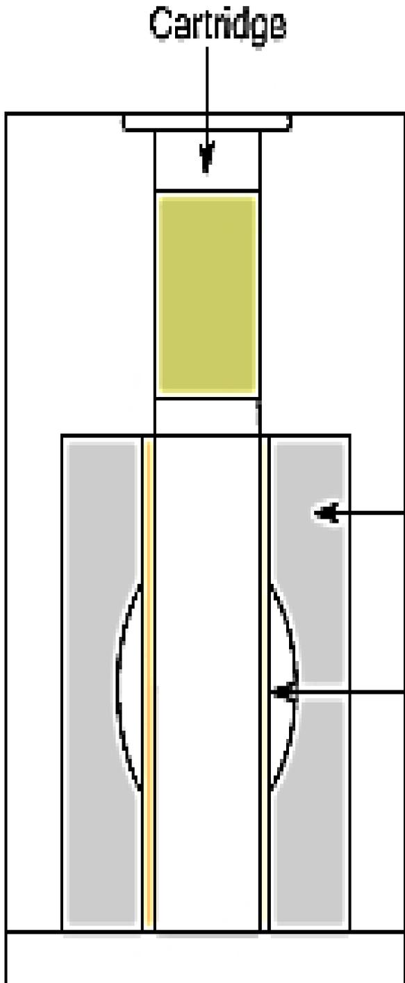
Schematic illustration of contact technique of explosive forming.
