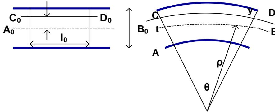
For our analysis, it may be assumed that a plane normal section in the sheet will remain plane and normal and converge on the center of curvature as shown in Figure. The line  $A_0B_0$  at the middle surface may change its length to  $AB$ , if the sheet is under stretching during bending. The original length  $l_0$  becomes,  $l_s = \rho\theta$ . A line  $C_0D_0$  at a distance  $y$  from the middle surface will deform to a length,
