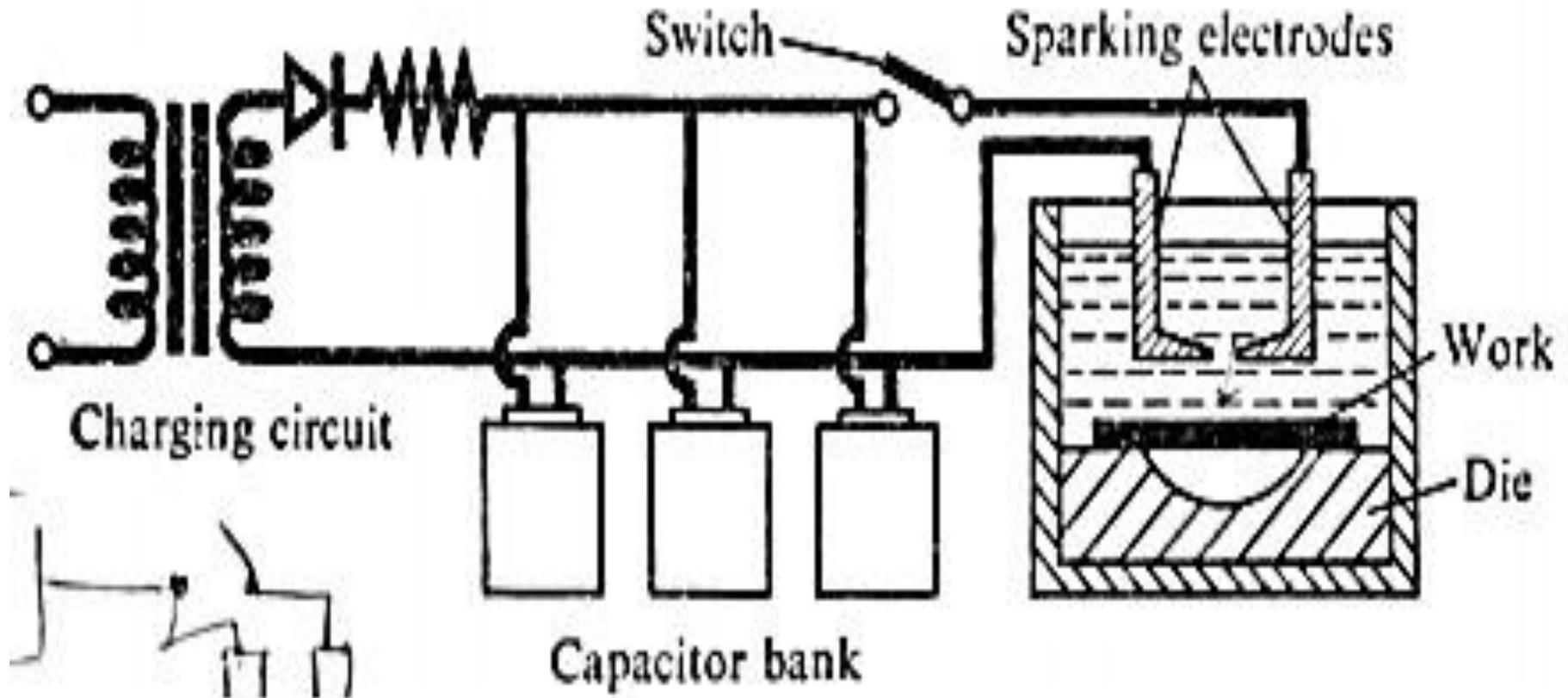
Fig. Electro Hydraulic Forming
