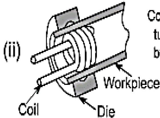
Coil inserted inside tube surrounded by die and insert
