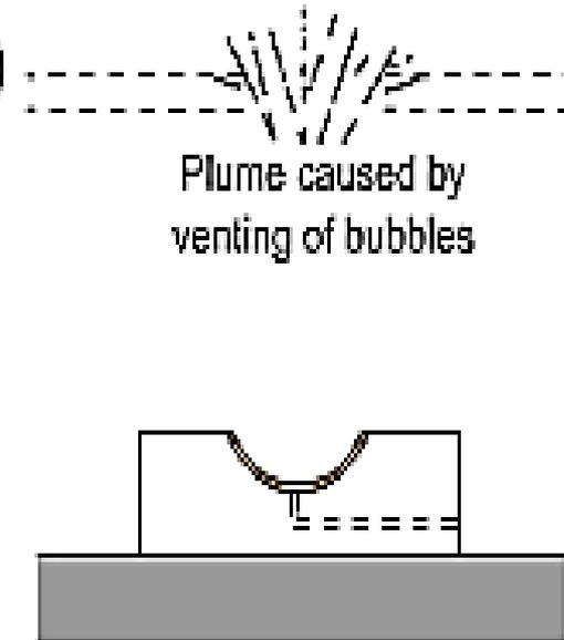
Sequeuce of underwater explosive forming operations.(i) explosive charge is set in position (ii) pressure pulse and gas bubble are formed as the detonation of charge occurs, (iii) workpiece is deformed, and (iv) gas bubbles vent at the surface of water.
