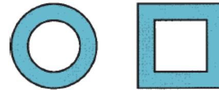
Making hollow shapes using direct extrusion
