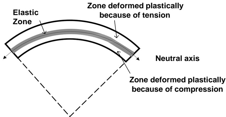
Elastic and plastic deformation zones during bending
