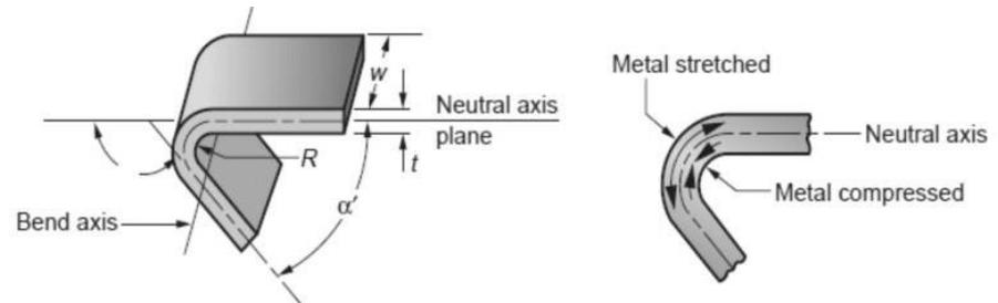
Bending can be seen as plane strain deformation as strain along bend can be zero
