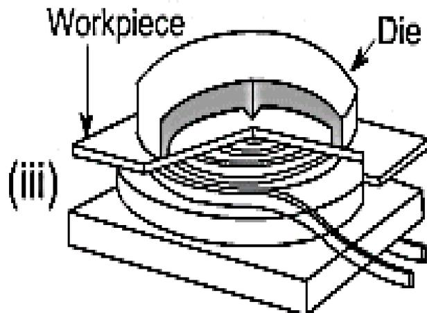
Coil placed under flat sheet with die on top
