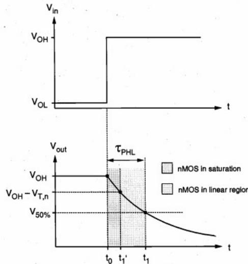
Fig. Input and output voltage waveforms during high-to-low transition.
