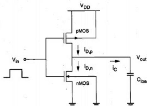
Fig. First-stage CMOS inverter with lumped output load capacitance.
