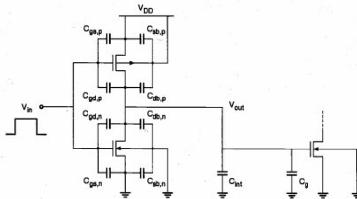
Fig. Cascaded CMOS inverter stages
