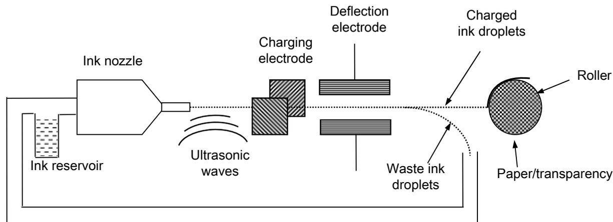
**Schematic of continuous flow inkjet printer**
