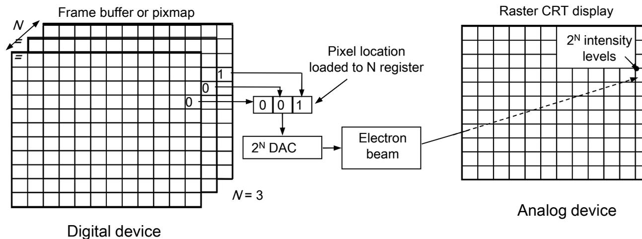
**N-bit-plane Monochrome gray level frame buffer raster CRT display**
