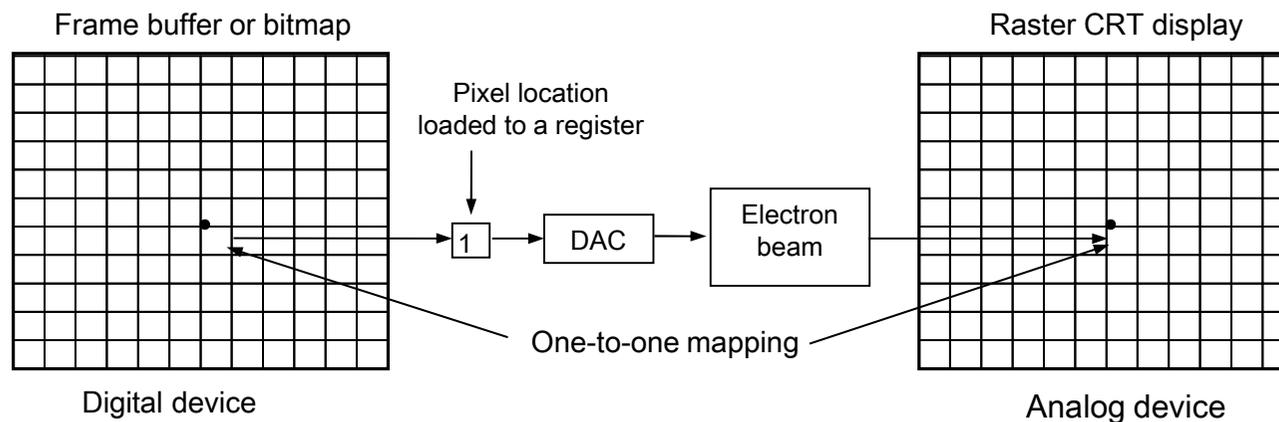
**Single-bit-plane monochrome frame buffer raster CRT display**
