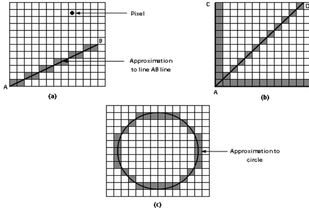
**Line (AB), special lines (AB, AC & AD) and circle, respectively, visible on the screen during rasterization.**
