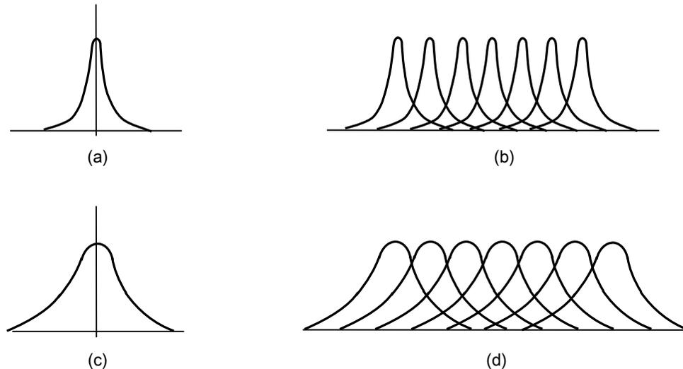
**Effect of cross-sectional intensity on resolution (a) Spot with well defined edges (b) Several such overlapping spots (c) Wider spot with less height (d) Several wider overlapping spots**
