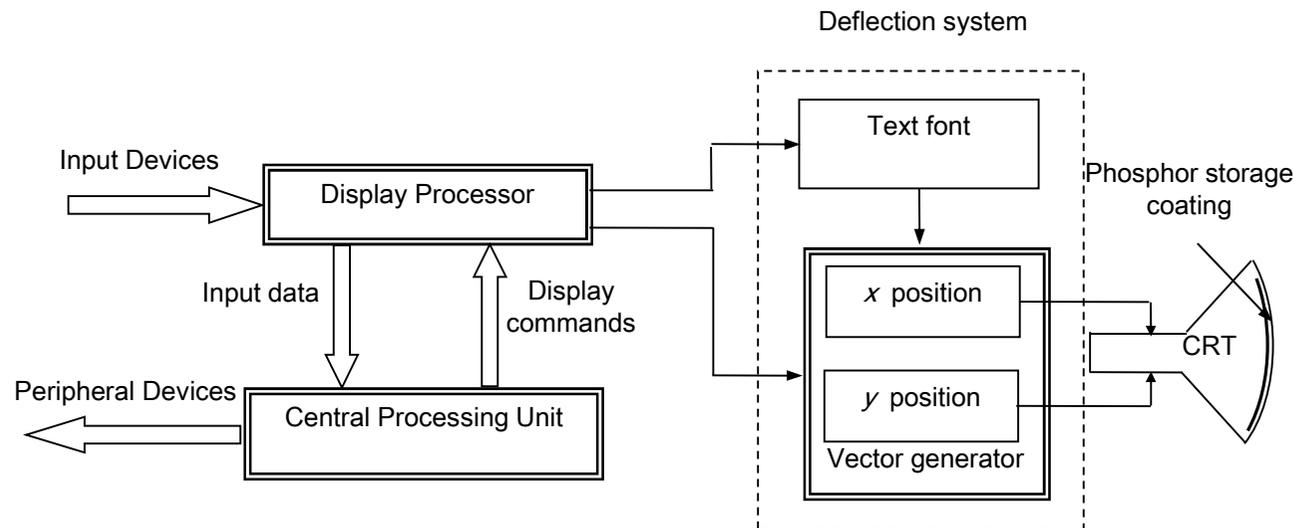
DVST Display System (Display file is missing)
