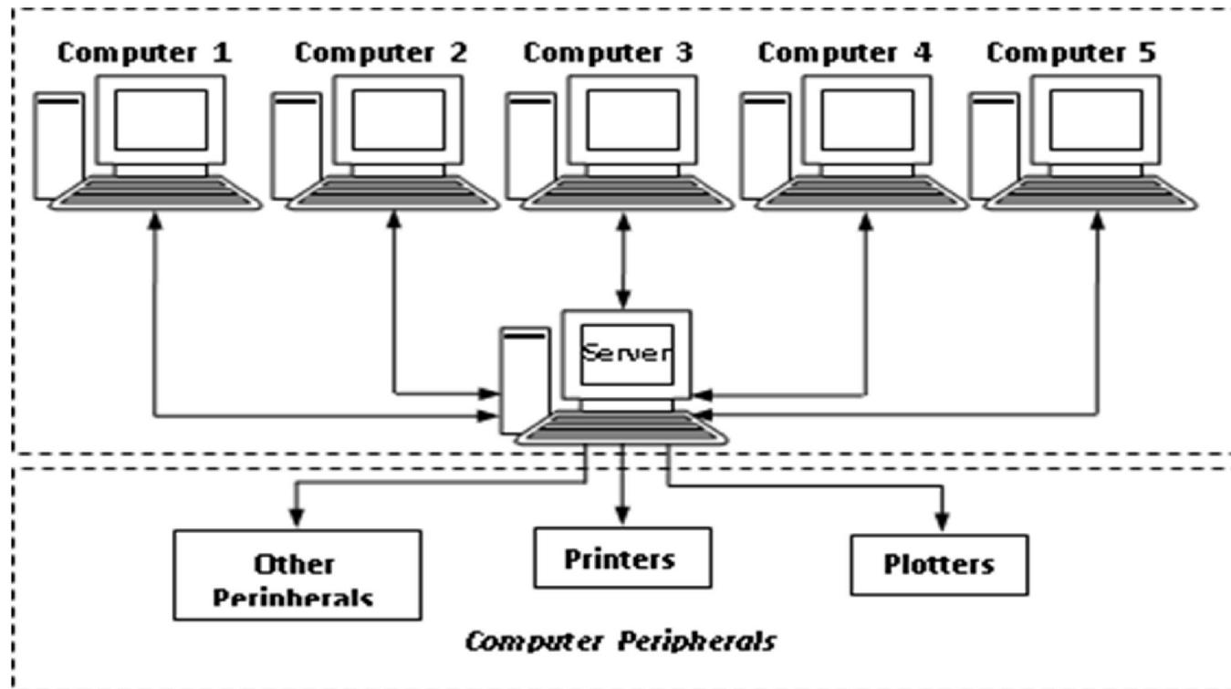
The workstation-based system has the advantages of distributed computation and networking potential with low cost as compared with the mainframe graphics system.
