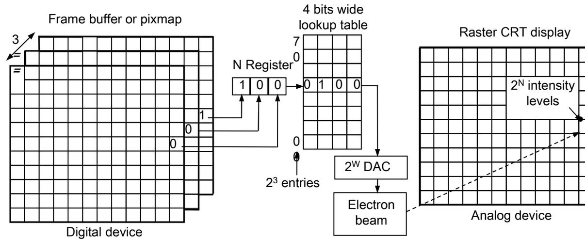
**A 3-bit-plane monochrome gray level frame buffer with 4-bits wide lookup table**
