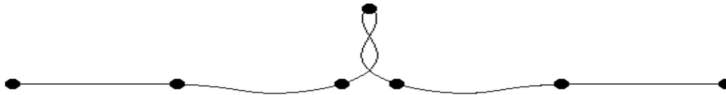
Interpolation Curve – over constrained → lots of (undesirable?) oscillations
