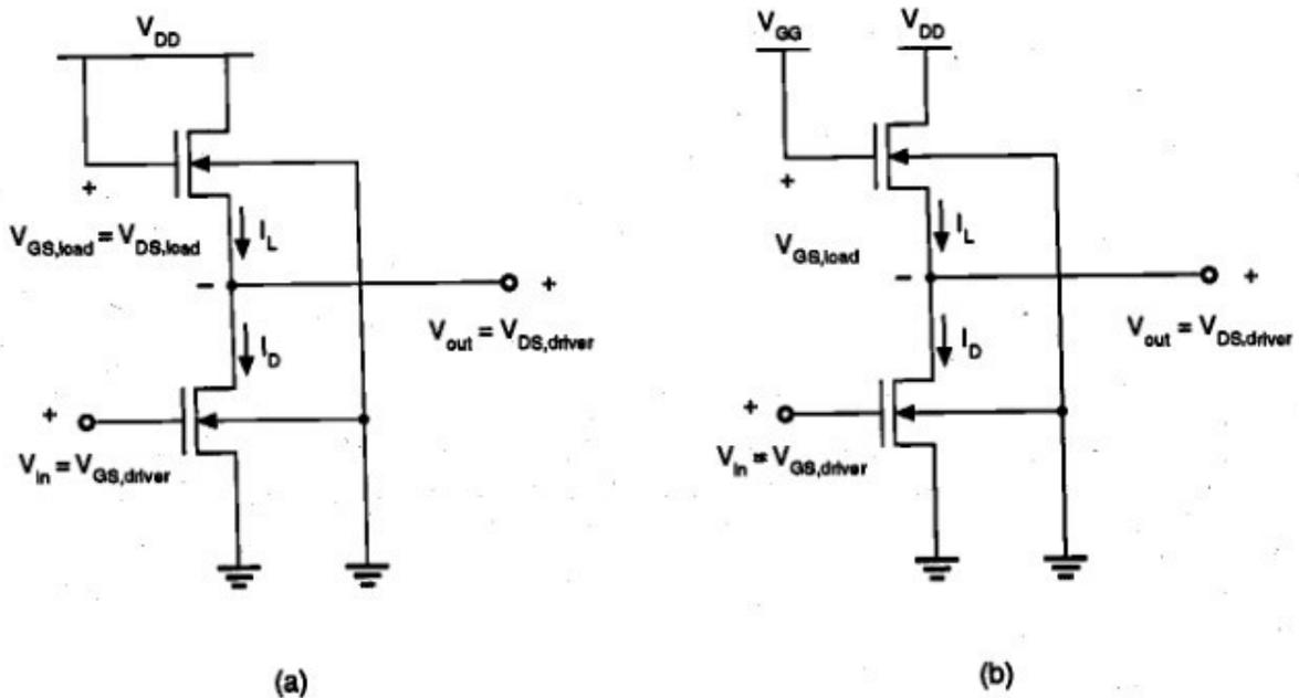
(a) Inverter circuit with saturated enhancement-type nMOS load. (b) Inverter with linear enhancement-type load.
