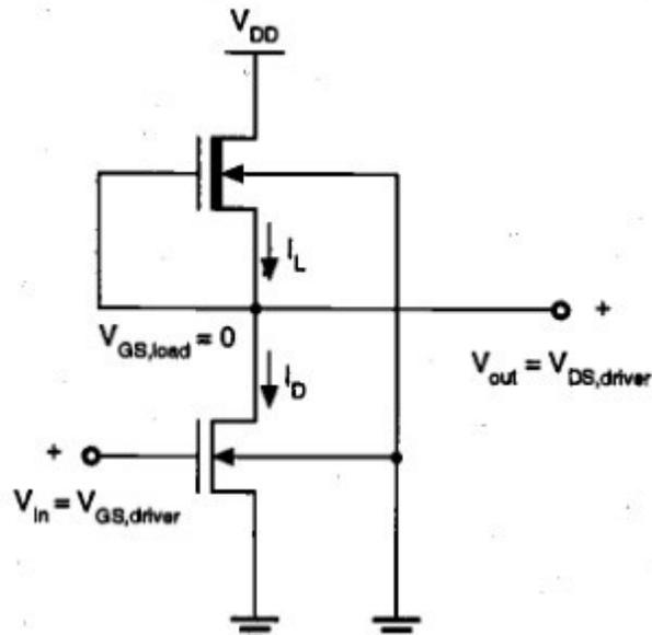
Several of the disadvantages of the enhancement-type load inverter can be avoided by using a depletion-type nMOS transistor as the load device.-The fabrication process for producing an inverter with an enhancement-type nMOS driver and a depletion-type nMOS load is slightly more complicated and requires additional processing steps, especially for the channel implant to adjust the threshold voltage of the load device.
