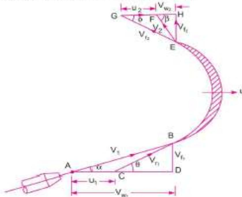
Fig. Jet striking a moving curved vane at one of the tips.
