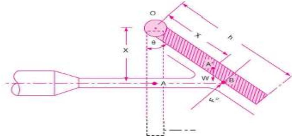
Fig. Force on a hinged plate.
