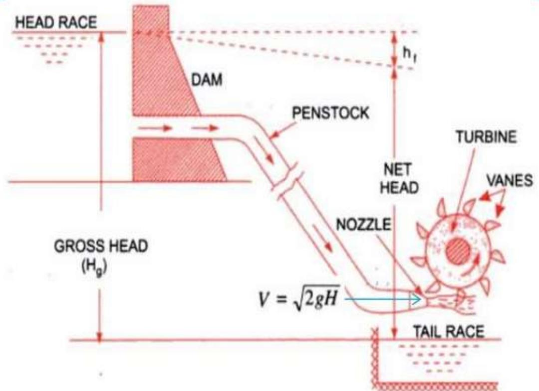
*Layout of a hydro-electric power plant.*
