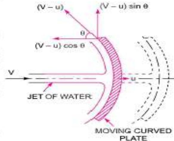
Fig. *Jet striking a curved moving plate.*
