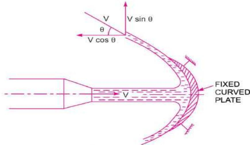
Fig. 3 Jet striking a fixed curved plate at centre.
