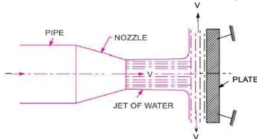
Fig. 1 Force exerted by jet on vertical plate.
