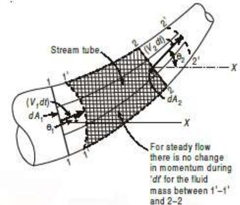
Figure 1 Change of momentum of fluid mass in flow passage
