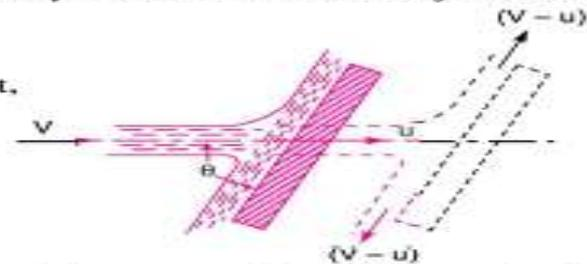
Fig. Jet striking an inclined moving plate.
