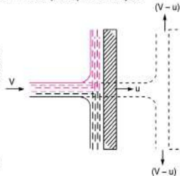
Fig. Jet striking a flat vertical moving plate
