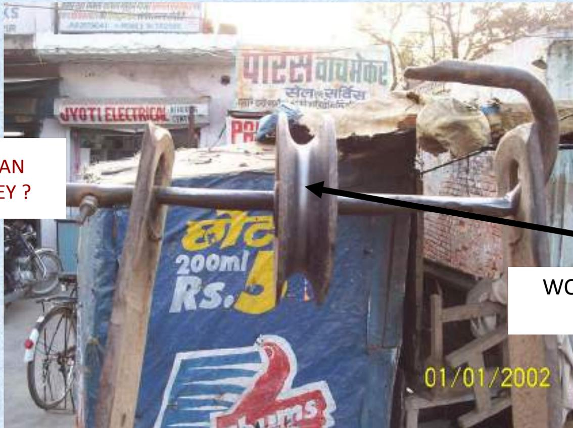
WORN OUT PULLEY BY A ROPE
