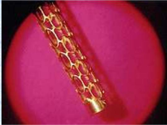
**LASER-CUT STENTLIKE PATTERN IN MINIATURE STAINLESS- STEEL TUBE WITH 1.25-mm OD.**
