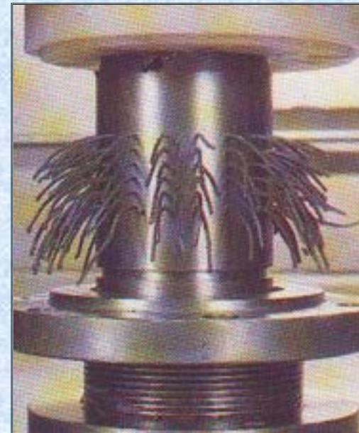
Abrasive Flow Machining (AFM) at IIT - K
