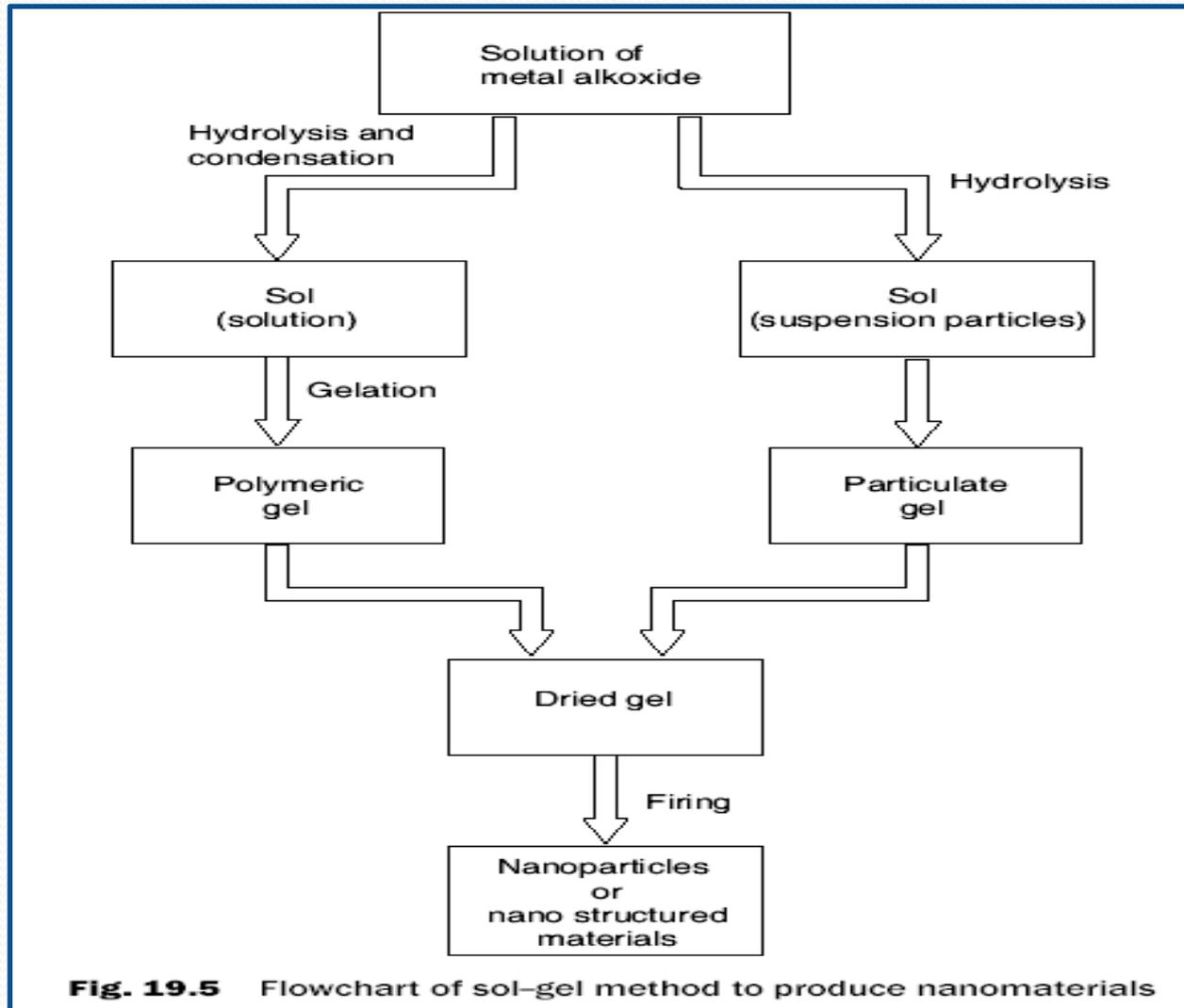
**Fig. 19.5** Flowchart of sol-gel method to produce nanomaterials
