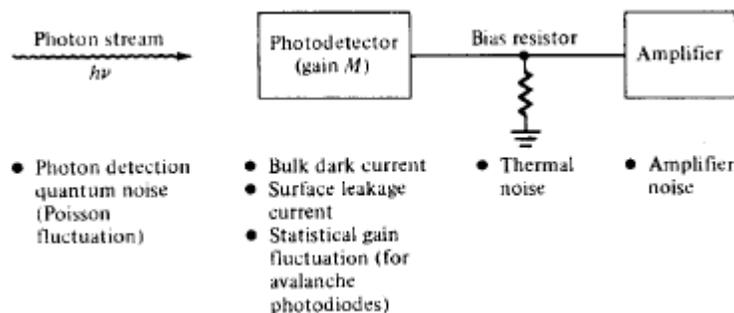
Errors in the detection mechanism can arise from various noises and disturbance associated with the signal distortion system.
