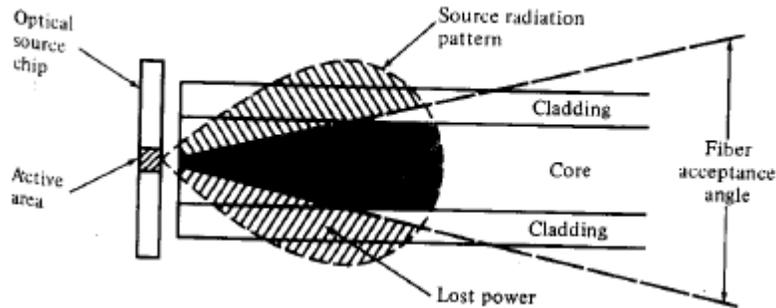
Here, the fiber end face is centered over emitting surface of the source and is positioned as close as possible.
