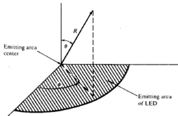
Here the figure shows a spherical coordinate system characterized by  $R$ ,  $\theta$  and  $\phi$  with the polar axis. The radiance may be a function of both  $\theta$  and  $\phi$  and can also vary from point to point on the emitting surface.
