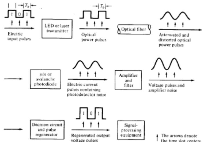
The transmitted signal is a two level binary data stream consisting of either a 0 or a 1 in a time slot of duration  $T_b$ . This time slot is referred to as a bit period. One technique for sending binary data is amplitude shift keying (ASK) or on-off key (OOK). The resultant
