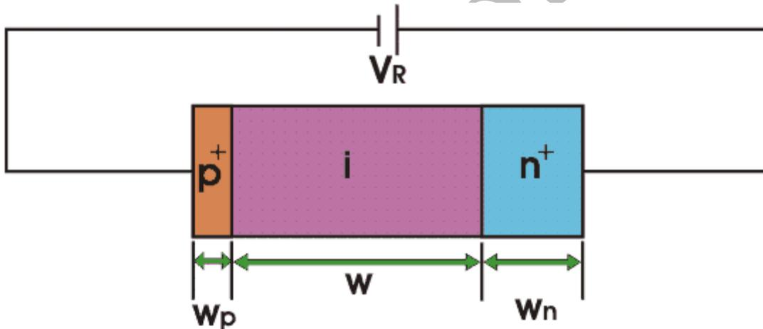
The most common semiconductor photo detector is the PIN photodiode.
