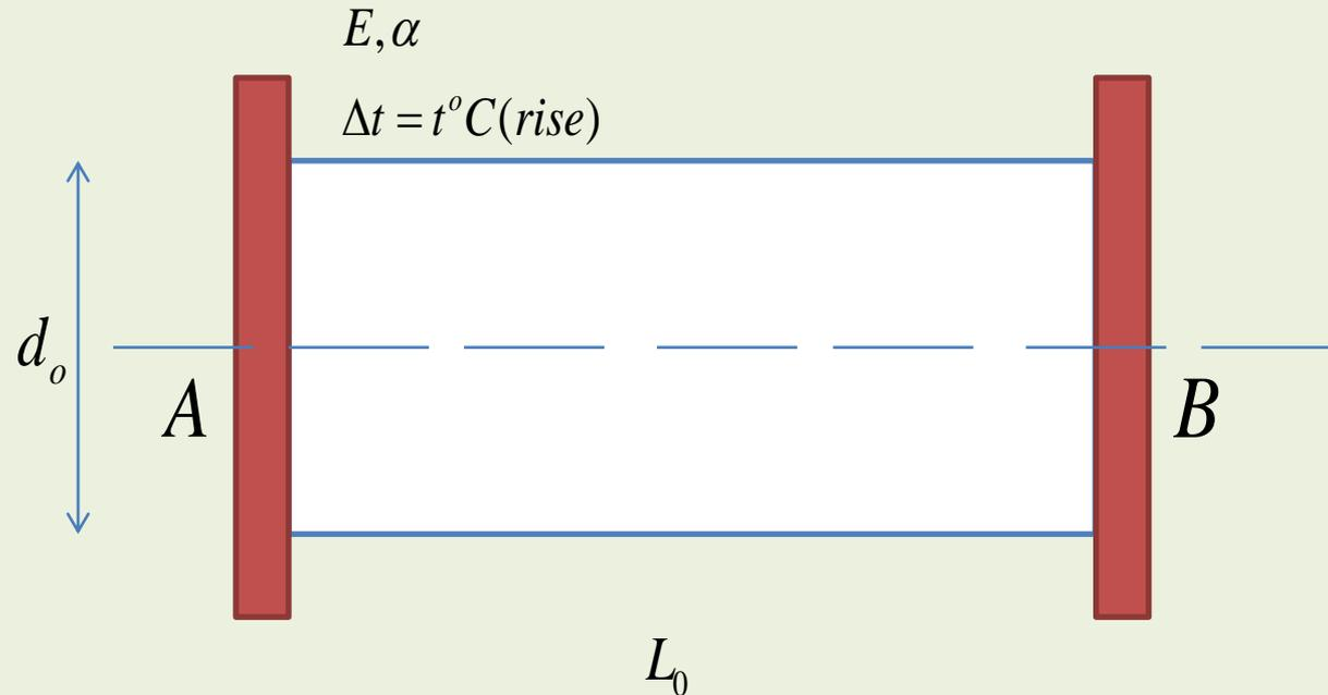
Fig. - A prismatic bar slightly held between two supports
