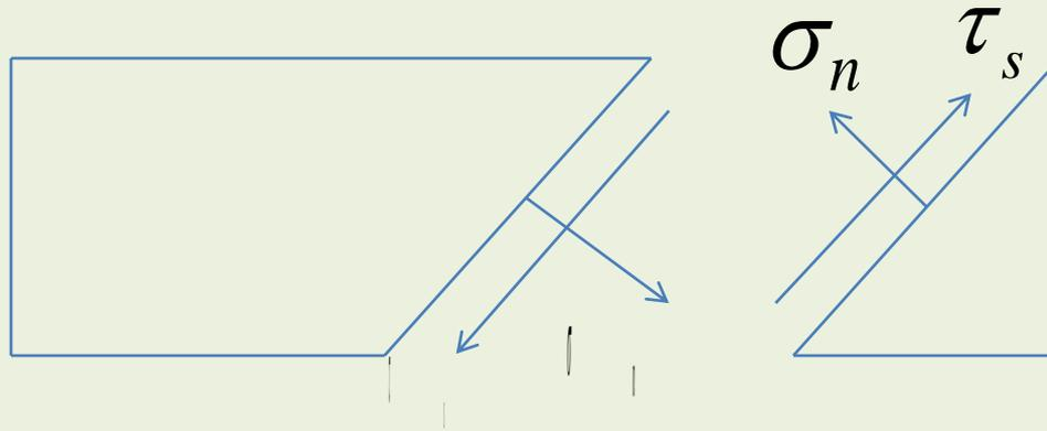
Shear stress on oblique plane is taken as positive when it forms a couple in anti-clockwise direction (ACW).
