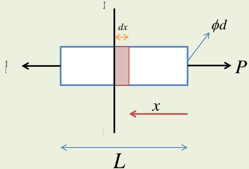
**General equation for strain energy when bar is subjected to pure axial load**
