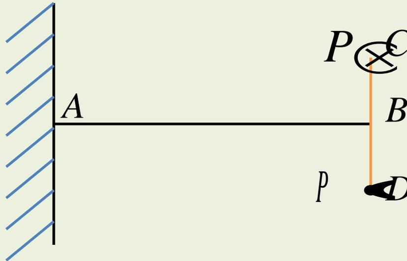
Q 3. For the given structure made of AB, BC & CD member. A external load  $P$  (N) is apply at the free end of member CD. Determine the which type of load (AL, TSL, ETSL, Bending & torsion) with respect to member AB, BC & CD.
