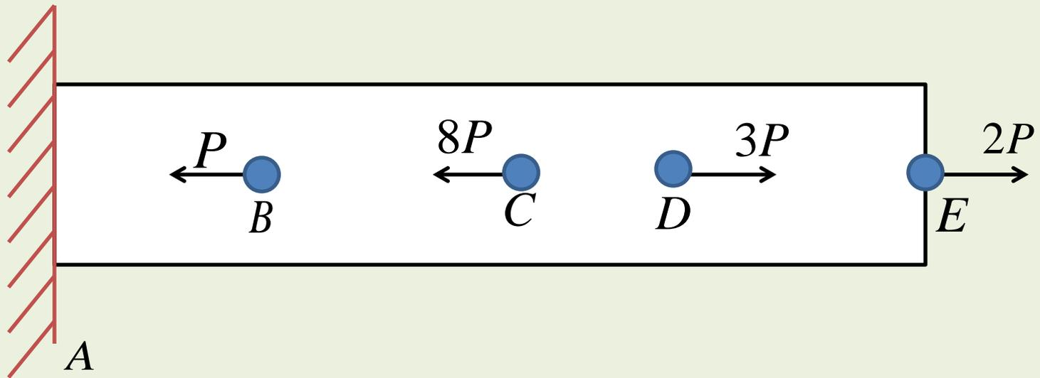
Q2. For the bar as shown in the figure determine the following maximum tensile load & maximum compressive load acting on the x-s/c of bar. Also determine the axial loads acting at the x-s/c A, B, C, D & E.
