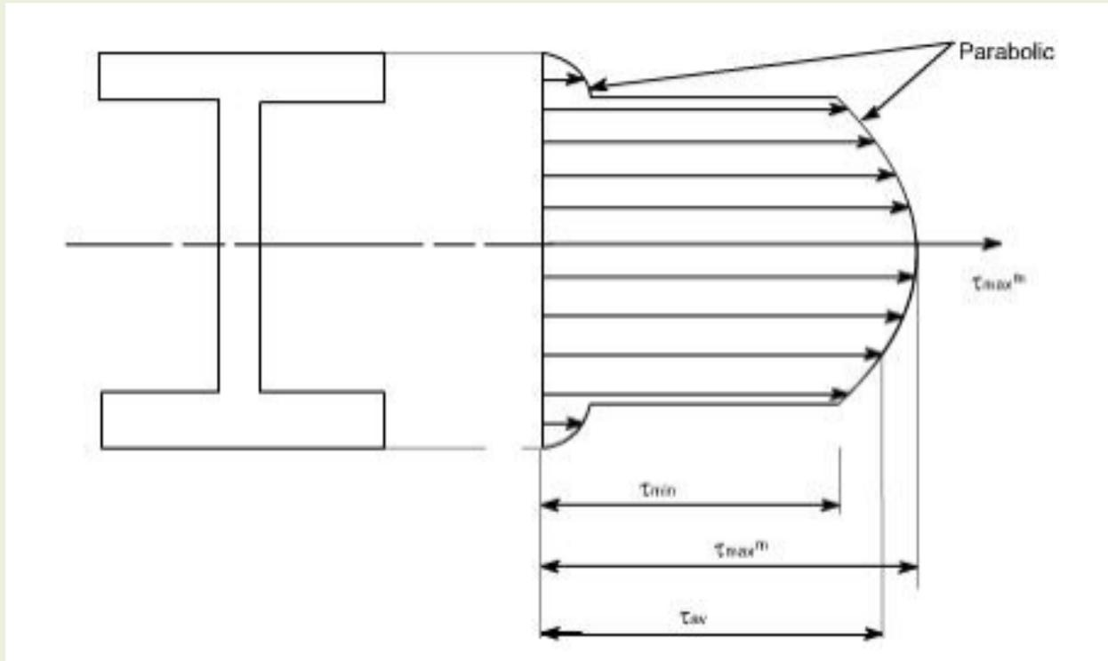
At the junction of web & flange, the section width change suddenly so there is drastically change in shear stress magnitude at web & flange junction.
