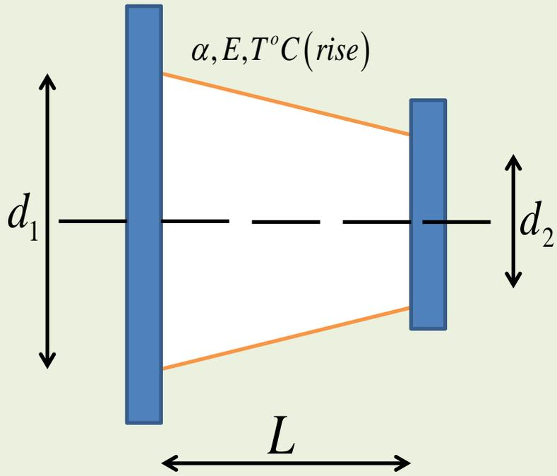
Q For the bar as shown in the fig. derive the expression for thermal stress.
