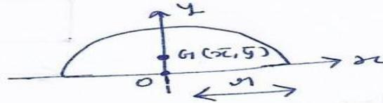
$$\begin{aligned} \text{Area} &= \frac{\pi r^2}{2} \\ \bar{x} &= 0 \\ \bar{y} &= \frac{4r}{3\pi} \end{aligned}$$
