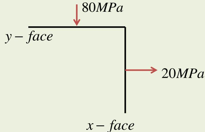
Q. Draw the Mohr's circle for a given state of stress of a point & determine the followings:
