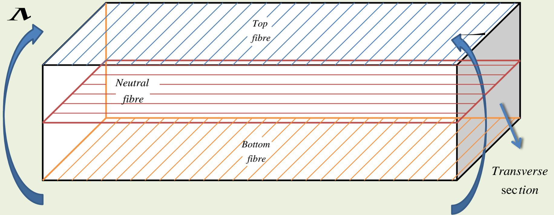
Figure: Type of sagging bending
