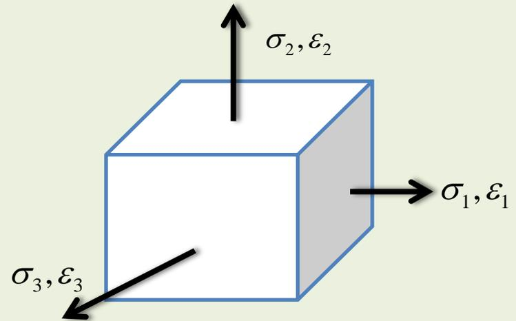
$$\frac{DE}{Vol^m} = \frac{1}{2E} \left[ (\sigma_1^2 + \sigma_2^2 + \sigma_3^2) - 2\mu(\sigma_1 \cdot \sigma_2 + \sigma_2 \cdot \sigma_3 + \sigma_3 \cdot \sigma_1) \right] - \frac{(1-2\mu)}{6E} \cdot (\sigma_1 + \sigma_2 + \sigma_3)^2$$
