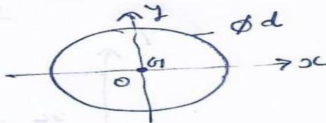
$$\begin{aligned} \text{Area} &= \frac{\pi}{4} d^2 \\ \bar{x} &= 0 \\ \bar{y} &= 0 \end{aligned}$$
