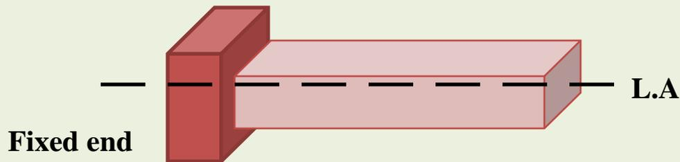
**Figure- Cantilever beam (one end is fixed & one end is free)**
