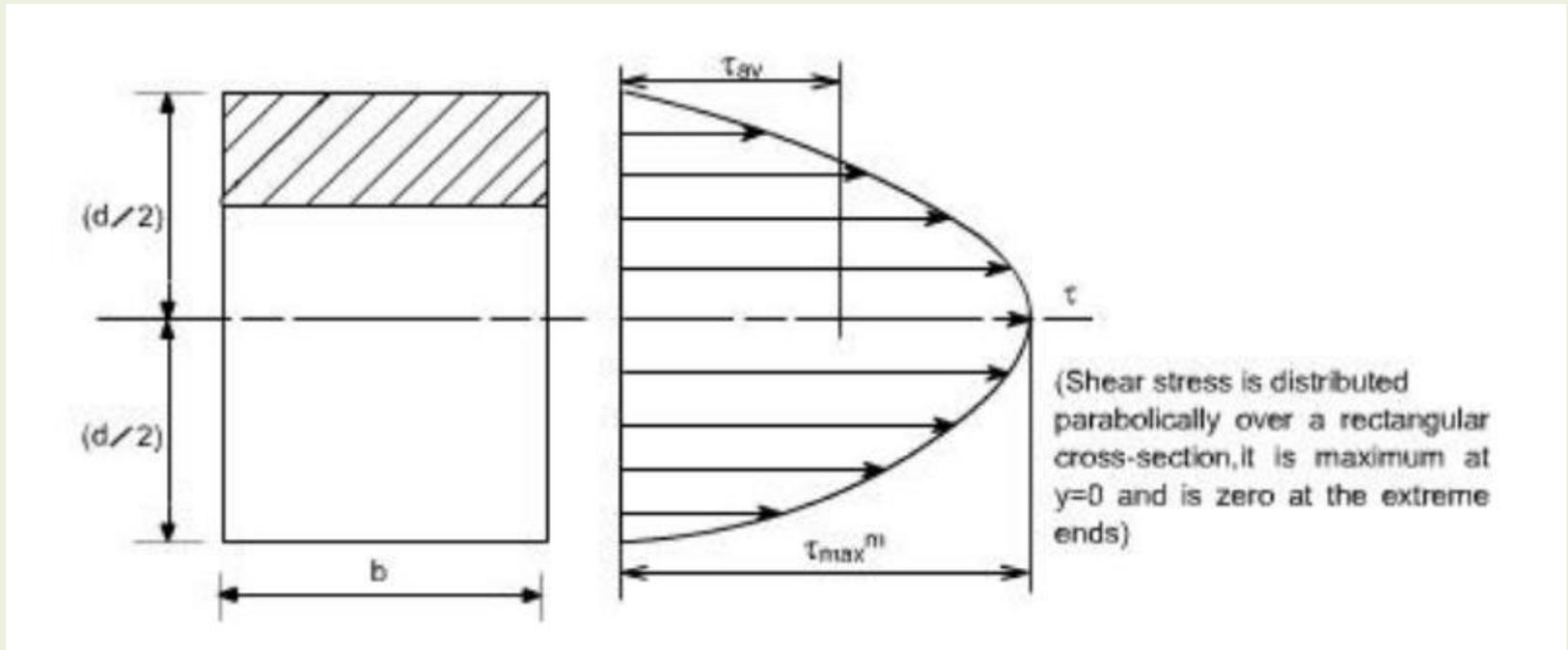
It may be noted that the shear stress is distributed parabolically over a rectangular cross-section, it is maximum at  $y = 0$  and is zero at the extreme ends.
