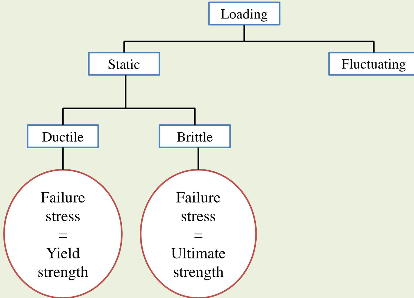
**Q. A component is made of brittle material having ultimate strength 350 MPa & yield strength 220 MPa. If the component is subjected a tensile force 150 N & having cross-section area 1 mm \* 1 mm. calculate factor of safety and margin of safety.**
