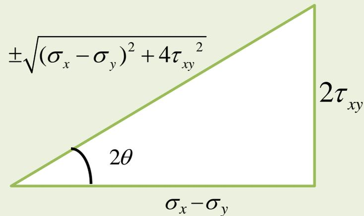
Substitute the value of  $\sin 2\theta$  &  $\cos 2\theta$  in normal stress ( $\sigma_n$ ) on oblique plane equation and we get the principal stresses  $\sigma_1$  &  $\sigma_2$  value in biaxial state of stress condition.
