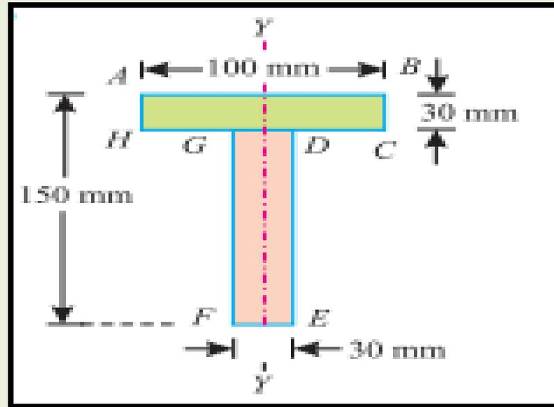
Note : If section is having symmetry about any axis, its centroid will lie on the symmetrical axis.
