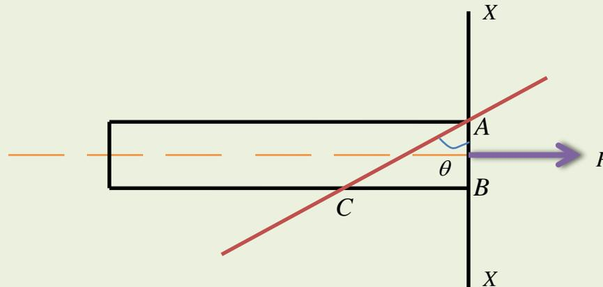
**State of stress:** It is representation of all the normal stresses ( $\sigma$ ) & shear stresses ( $\tau$ ) acting at a point in a material in all the three mutual perpendicular directions.
