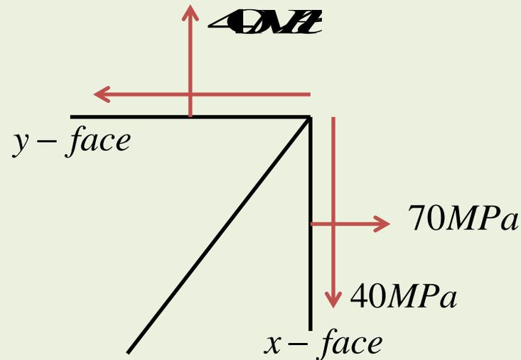
Q. At a point in a material subjected to 2 direct stresses on a plane at right angle. The resultant stress on a plane A is 80 MPa and inclined at  $30^\circ$  to the normal stress and the resultant stress on a plane B is 40 MPa which is inclined to  $45^\circ$  to the normal stress. Find the principal stresses & show the position of two planes A & B relative to the principal plane.
