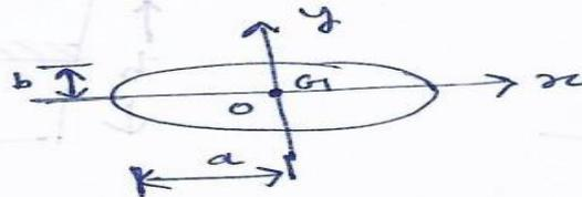
$$\begin{aligned} \text{Area} &= \pi ab \\ \bar{x} &= 0 \\ \bar{y} &= 0 \end{aligned}$$
