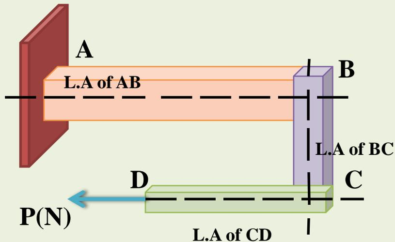
Q 2. For the given structure made of AB, BC & CD member. A external load  $P$  (N) is apply at the free end of member CD. Determine the which type of load (AL, TSL & ETSL) with respect to member AB, BC & CD.
