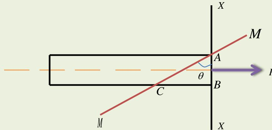
Consider a oblique plane M-M, cut at an angle  $\theta$  in clockwise direction from the x-sectional plane X-X.
