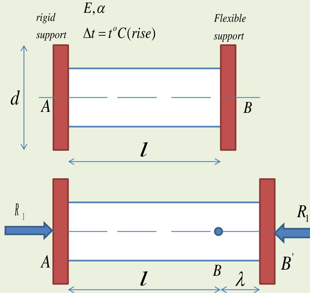
$R_1$  = Reaction offered by flexible support like spring.
