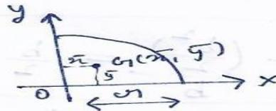
$$\begin{aligned} \text{Area} &= \frac{\pi r^2}{4} \\ \bar{x} &= \frac{4r}{3\pi} \\ \bar{y} &= \frac{4r}{3\pi} \end{aligned}$$
