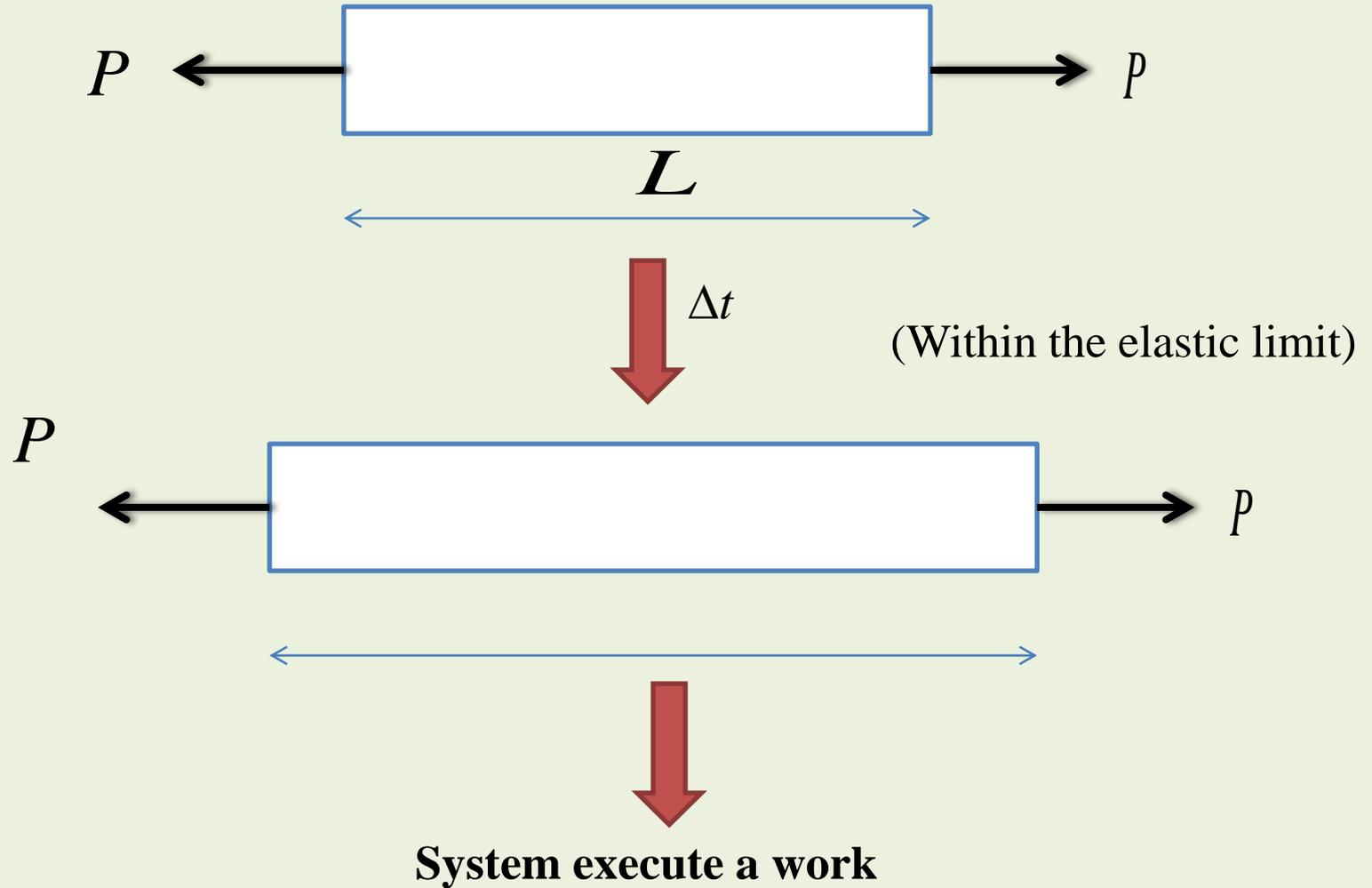
This work is stored within the body in form of internal energy
