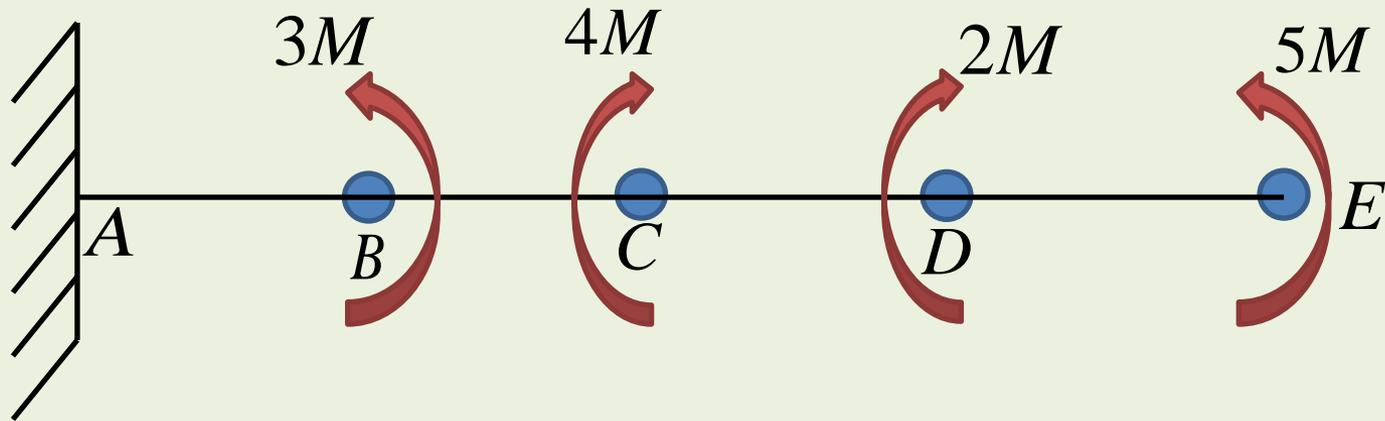
Q2. For the S.S.B as shown in the figure draw the bending moment diagram. Determine maximum sagging and maximum hogging bending moment acting at the x-s/c of the beam.
