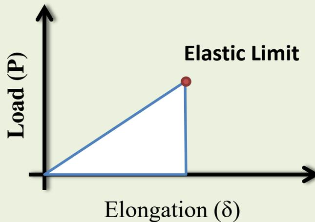
$U = \text{Area under (P-}\delta\text{) curve}$
