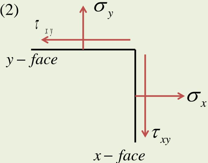
3. Locate a point A corresponding to the state of stress on x-face.
