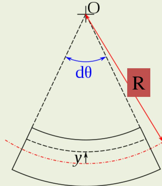
**Neutral Fibre** : All the fibre that lengths get unchanged before and after the bending, is said to be neutral fibre.
