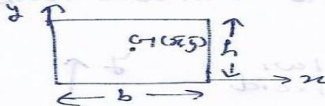
$$\begin{aligned} \text{Area} &= b \times h \\ \bar{x} &= b/2 \\ \bar{y} &= h/2 \end{aligned}$$
