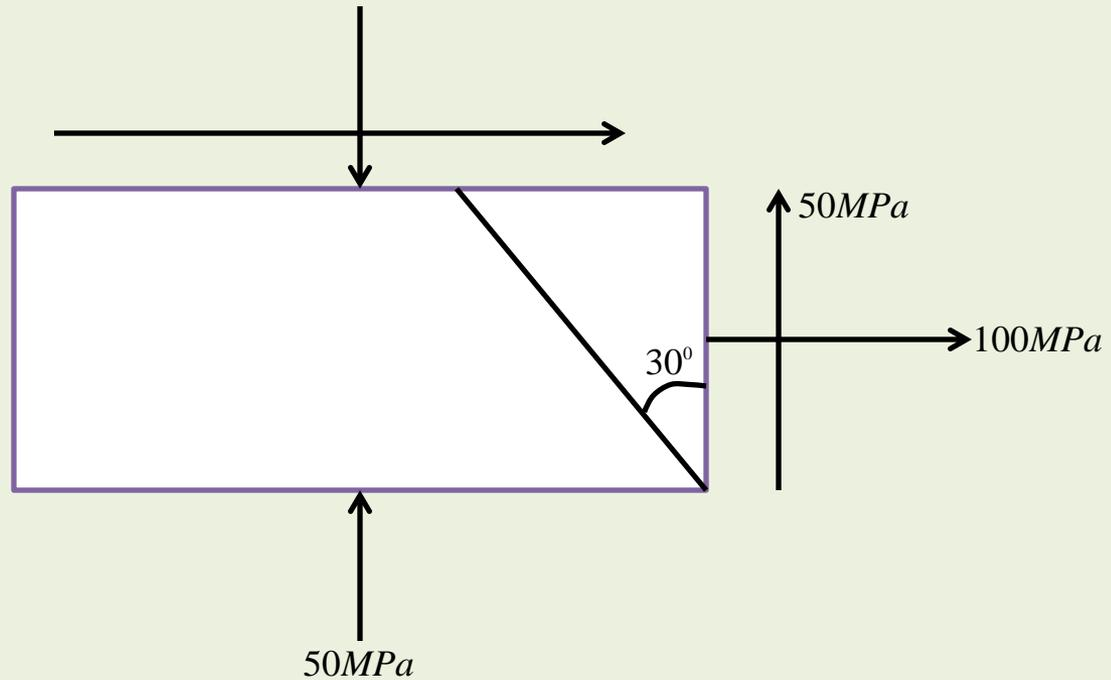
Q2. Determine the normal stress and shear stress on an oblique plane for a given state of stress.
