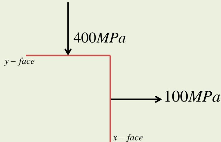
Q. for the given stress tensor at a point , determine the following -
