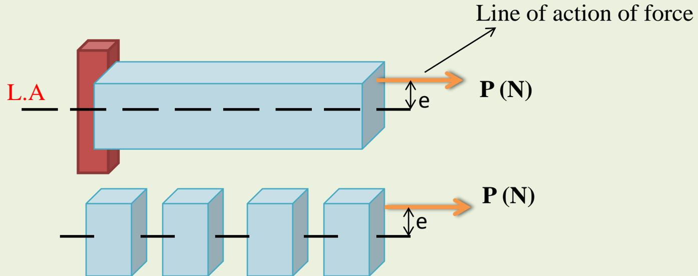
**Figure: Eccentric axial normal load**
