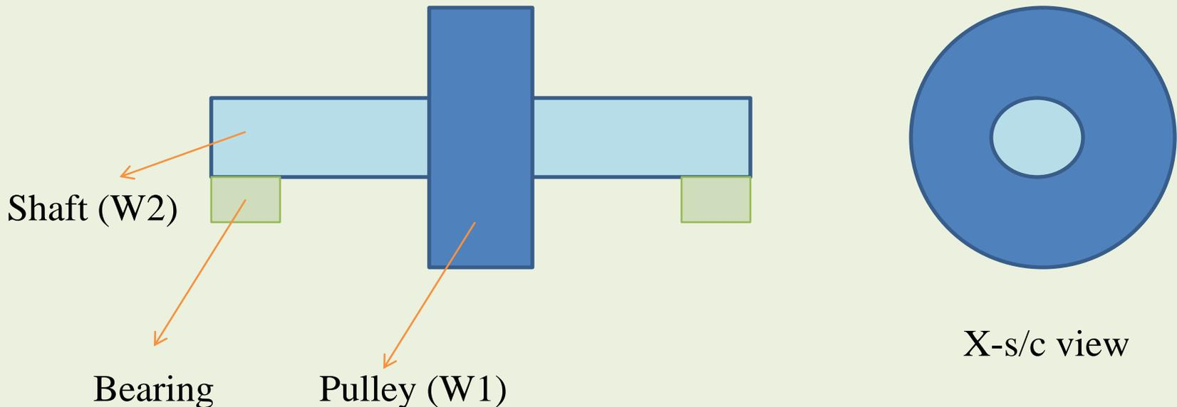
Fig. Shaft support a pulley & bearing's support shaft and pulley both
