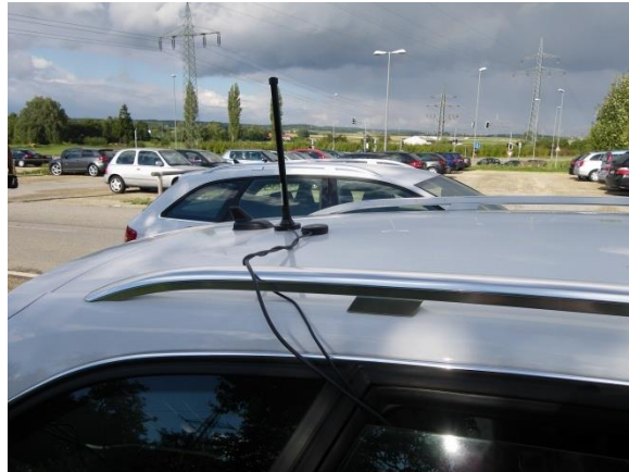
Fig. Omnidirectional Tx and GPS receiver mounted on a Car [1]
