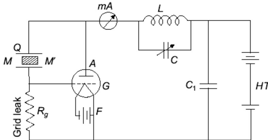
The natural frequency of quartz crystal of thickness  $t$  for its fundamental mode of vibration is given as
