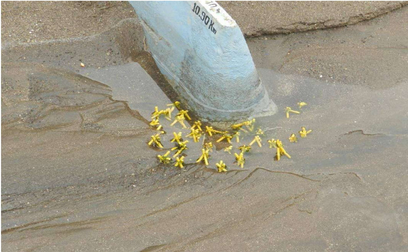
Typical photograph of dry model after running the model for a discharge of 5,663 m 3 /s with porcupine units placed near the spur nose.
