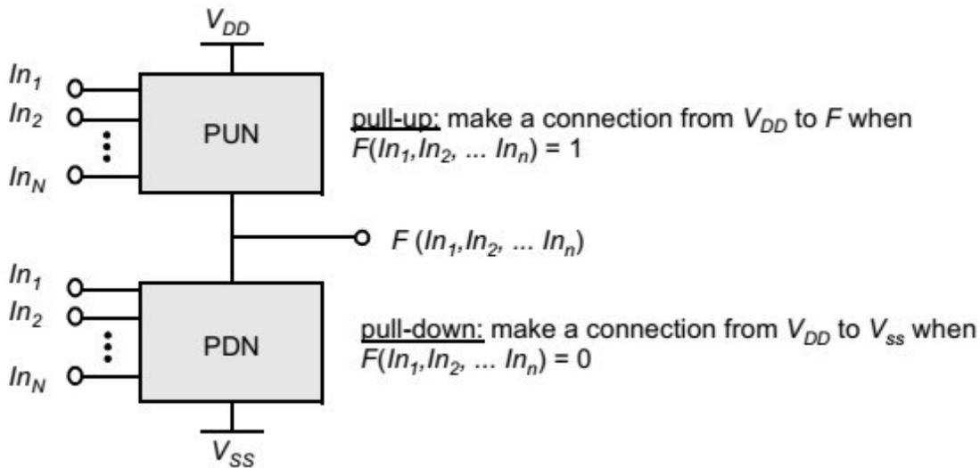
Complementary logic gate as a combination of a PUN (pull-up network) and a PDN (pull-down network)
