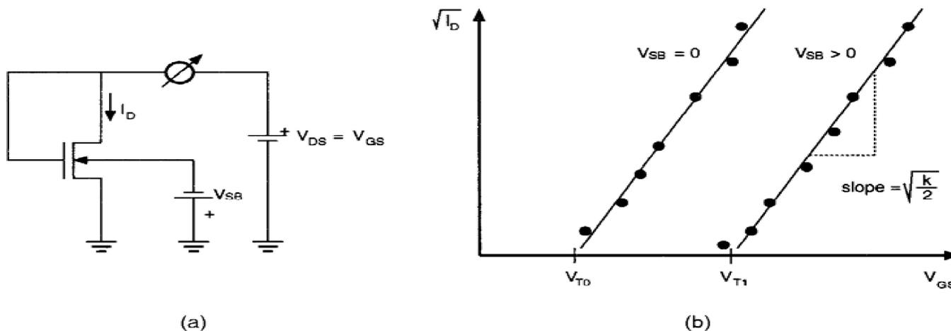
**Figure 3.22** (a) Test circuit arrangement and (b) measured data for experimental determination of the parameters  $k_n$ ,  $V_{T0}$ , and  $\gamma$ .
