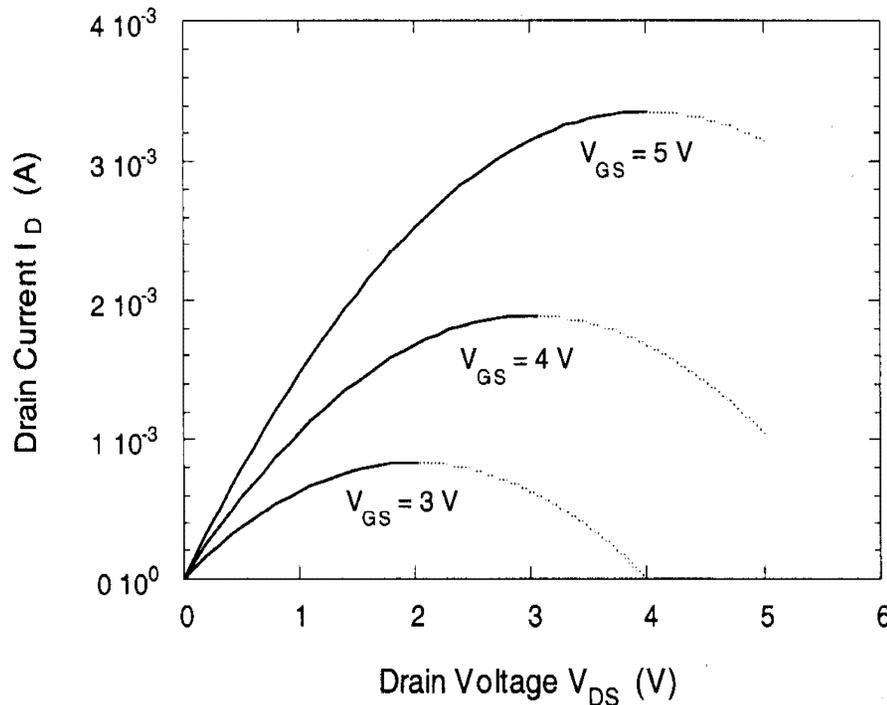
The drain current-drain voltage curves shown on page 104 reach their peak value for  $V_{DS} = V_{GS} - V_{T0}$ . Beyond this maximum, each curve exhibits a *negative* differential conductance, which is not observed in actual MOSFET current-voltage measurements (section shown by the dashed lines). We must remember now that the drain current equation (3.32) has been derived under the following voltage assumptions,
