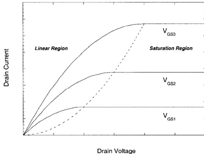
**Figure 3.17** Basic current-voltage characteristics of an n-channel MOS transistor.
