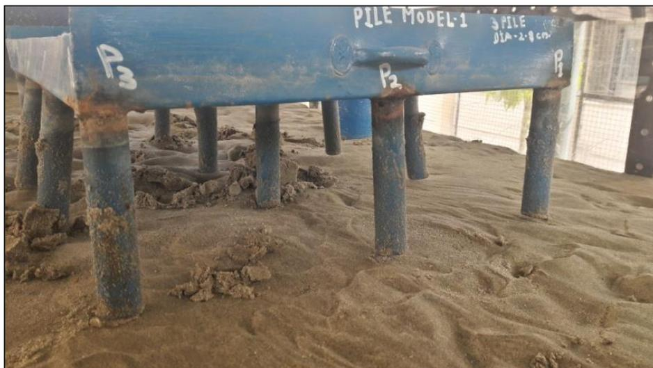
Fig.3.2 Experimental Composite foundation model
