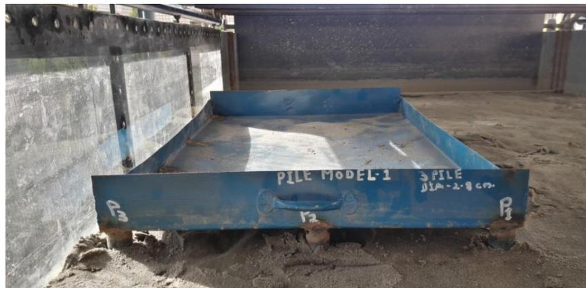
Figure: 3.6 Composite foundation Model near side wall of the channel
