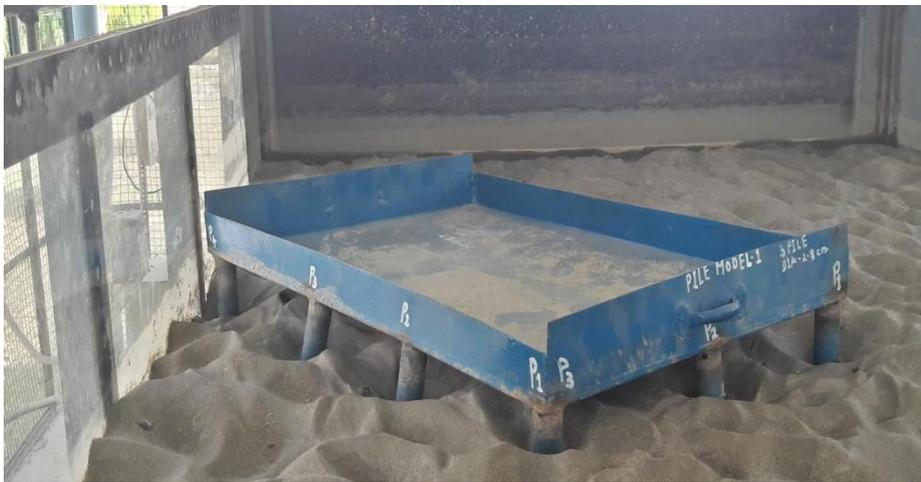
Figure: 3.11 Composite foundation Model Tilted by  $45^\circ$  w.r. to side face of the channel
