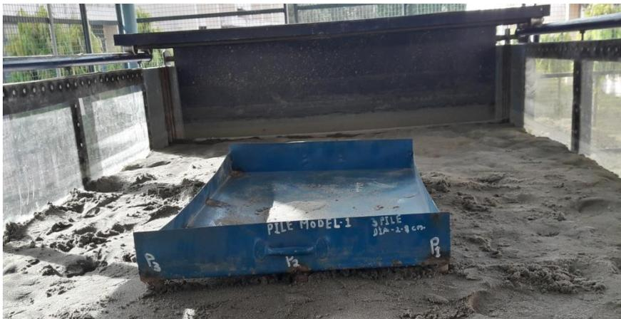
Figure: 3.8 Composite foundation Model placed 49.5cm away from side face of the channel
