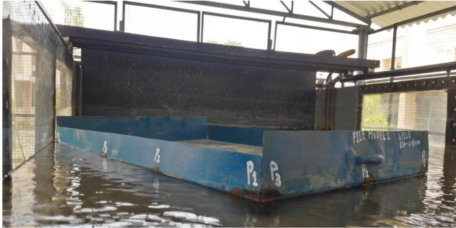
Figure: 3.10 Composite foundation Model Tilted by  $30^\circ$  w.r. to side Face of the channel
