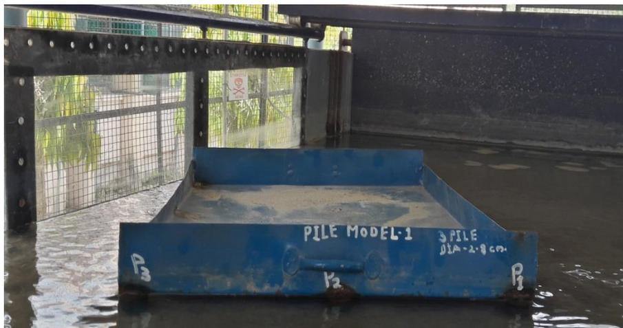
Figure: 3.9 Composite foundation Model Tilted by 15° w.r. to side Face of the channel
