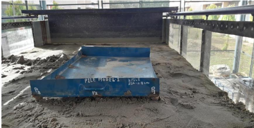
Figure: 3.7 Composite foundation model placed 30cm away from side face of the channel
