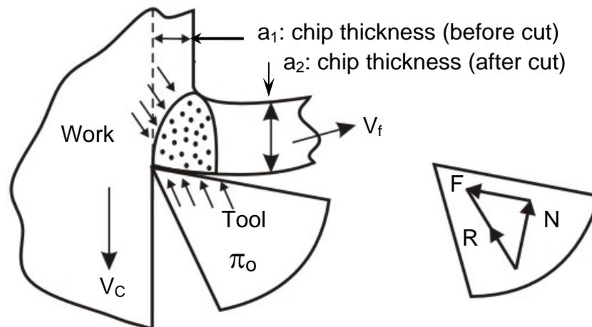
**Fig. 5.1** Compression of work material (layer) ahead of the tool tip
