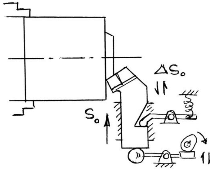
**Fig. 7.14** Dynamic chip breaking in radial operations in lathe.
