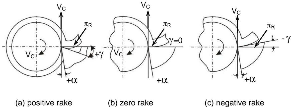
**Fig. 3.2** Three possible types of rake angles
