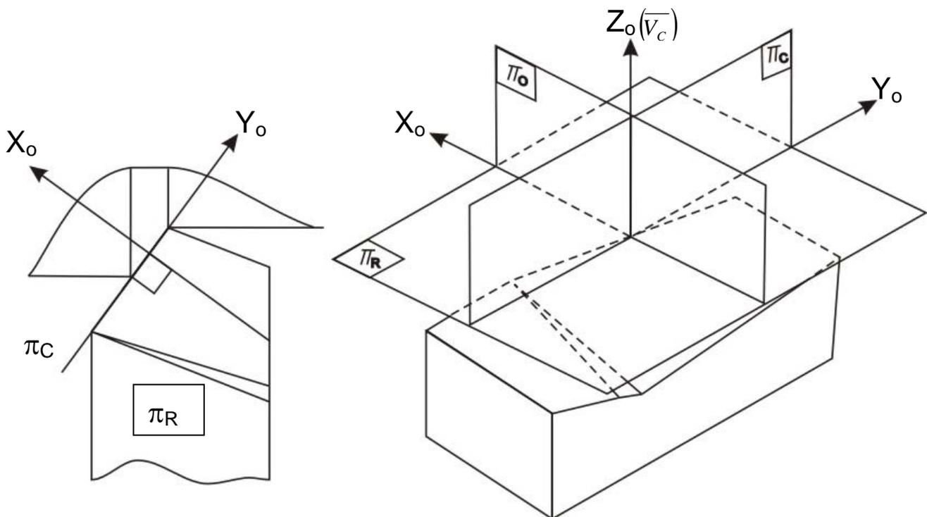
**Fig. 3.6** Planes and axes of reference in ORS
