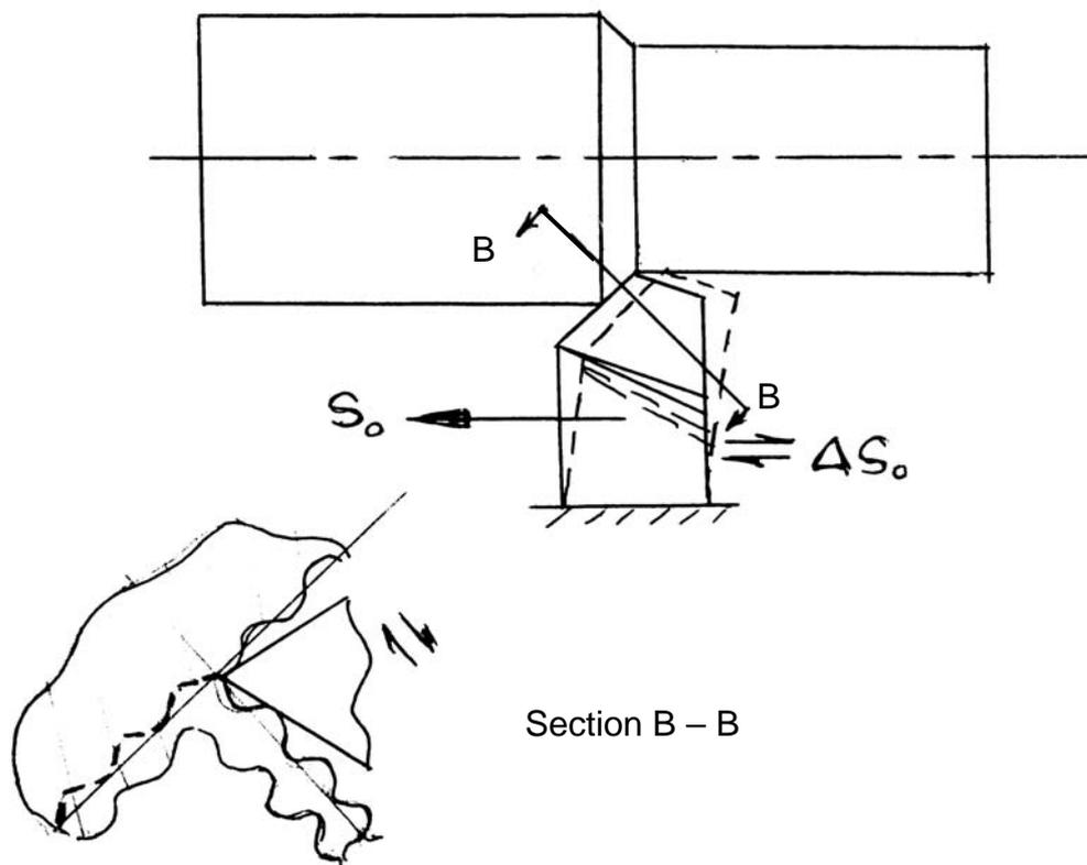
**Fig. 7.13** Self chip breaking in dynamic turning.
