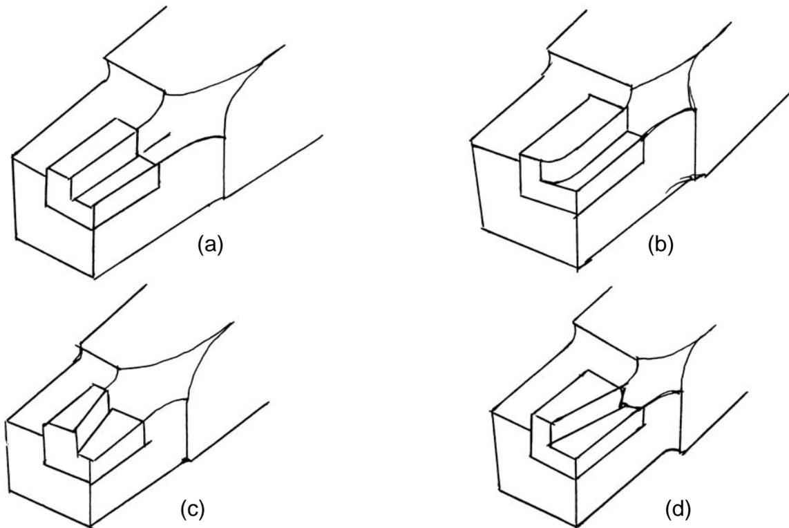
**Fig. 7.3** Step type in-built chip breaker (a) parallel step (b) parallel and radiused (c) positive angular (d) negative angular
