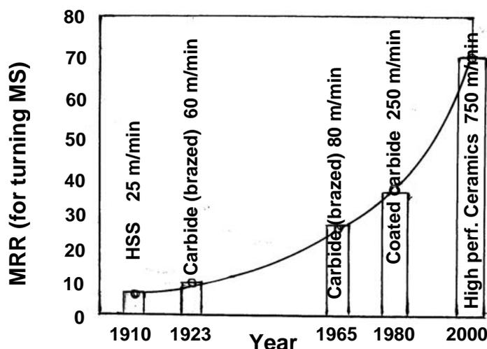
Fig. 3.3.1 Productivity raised by cutting tool materials.
