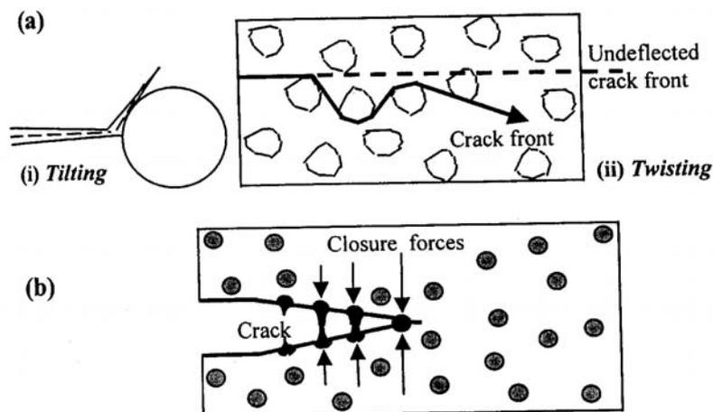
**Fig. 3.3.8** Toughening mechanism of alumina by metal dispersion.
