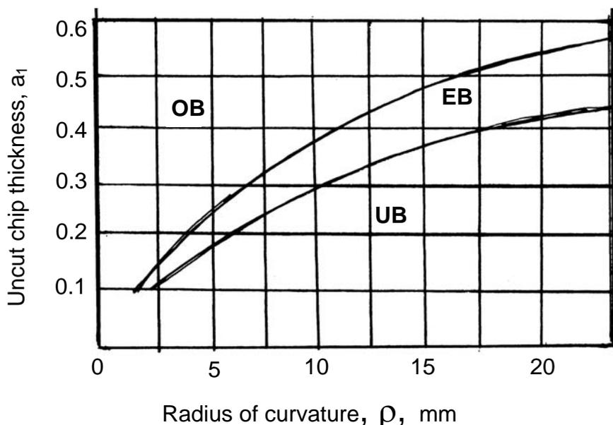
OB – over breaking, EB – effective breaking, UB – under breaking
