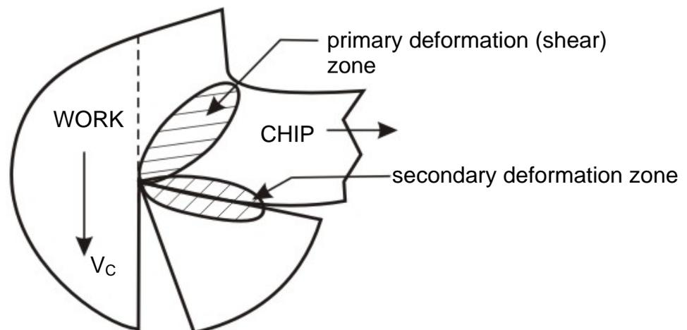
**Fig. 5.3** Primary and secondary deformation zones in the chip.
