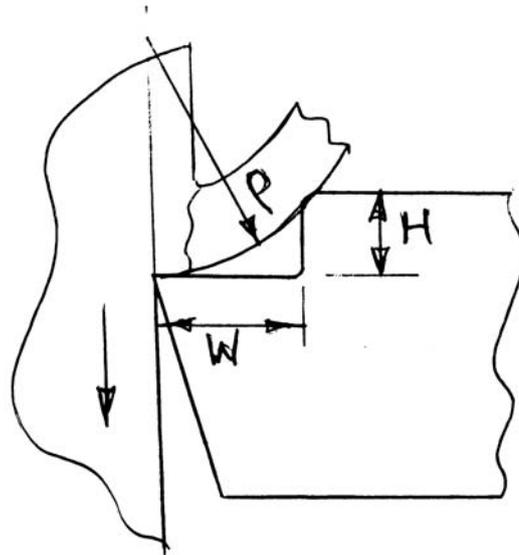
$W$  = width,     $H$  = height,     $\beta$  = shear angle
