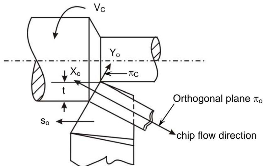
**Fig. 6.1** Ideal direction of chip flow in turning
