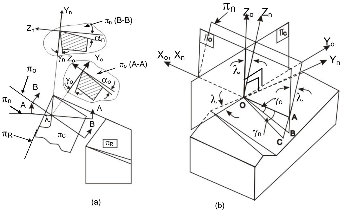
**Fig. 3.9** Differences of NRS from ORS w.r.t. cutting tool geometry.
