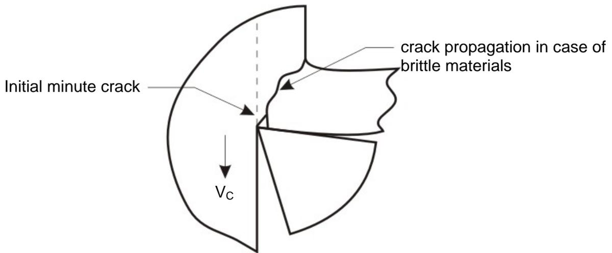
**Fig. 5.5** Development and propagation of crack causing chip separation.
