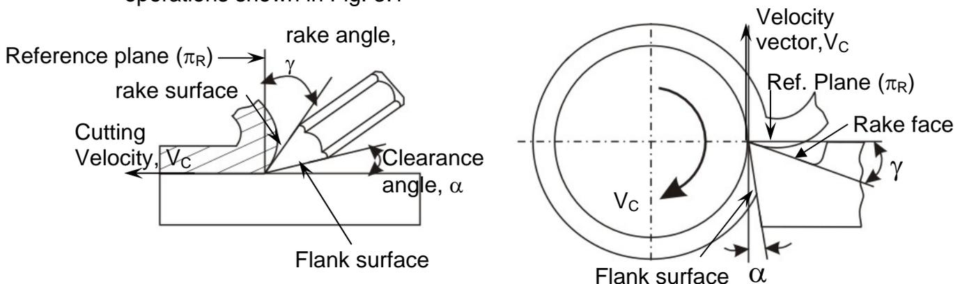
**Fig. 3.1** Rake and clearance angles of cutting tools.
