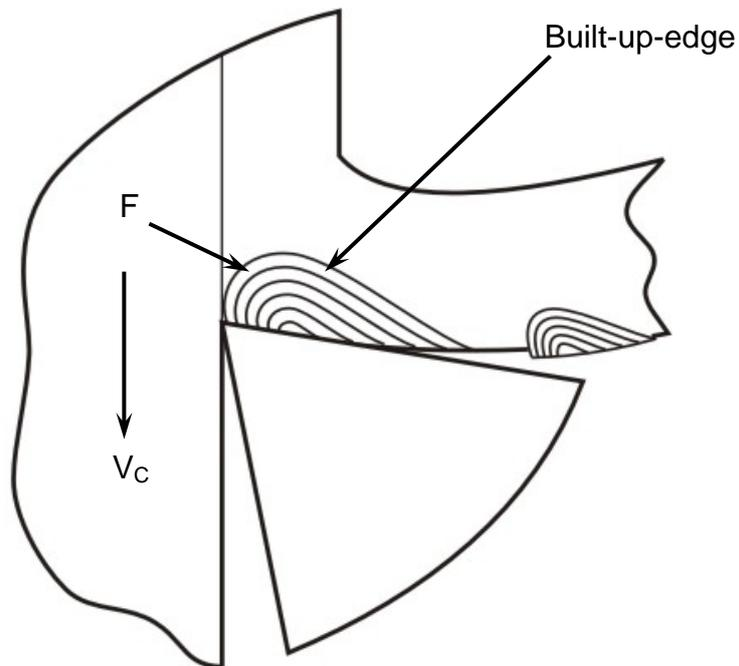
**Fig. 5.11** Scheme of built-up-edge formation
