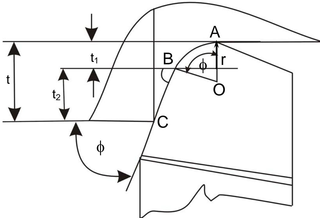
**Fig. 6.5** Variation of principal cutting edge angle in nose radiused tools.
