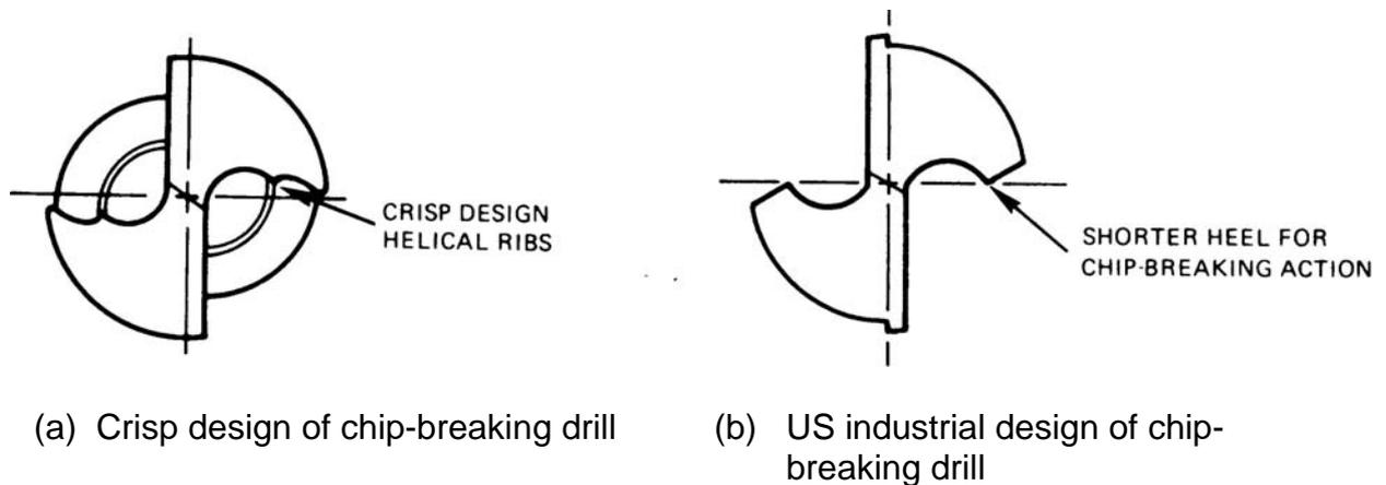
(a) Crisp design of chip-breaking drill
