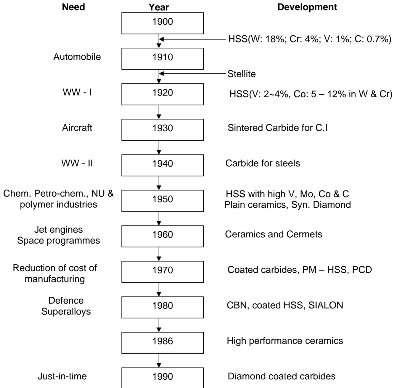
**Fig. 3.3.2** Chronological development of cutting tool materials.
