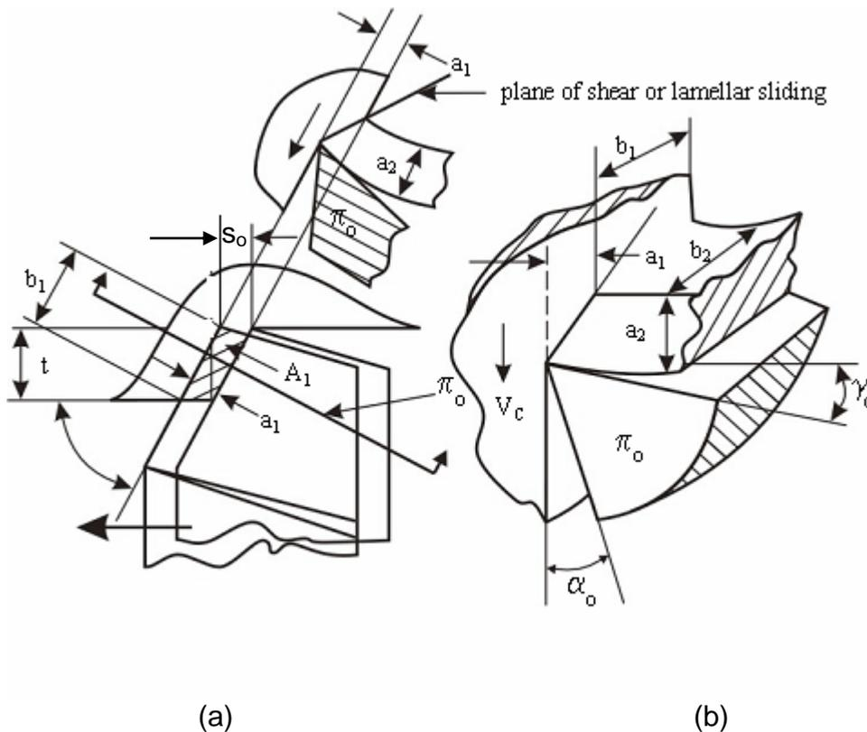
**Fig. 5.7** Geometrical features of continuous chips' formation.
