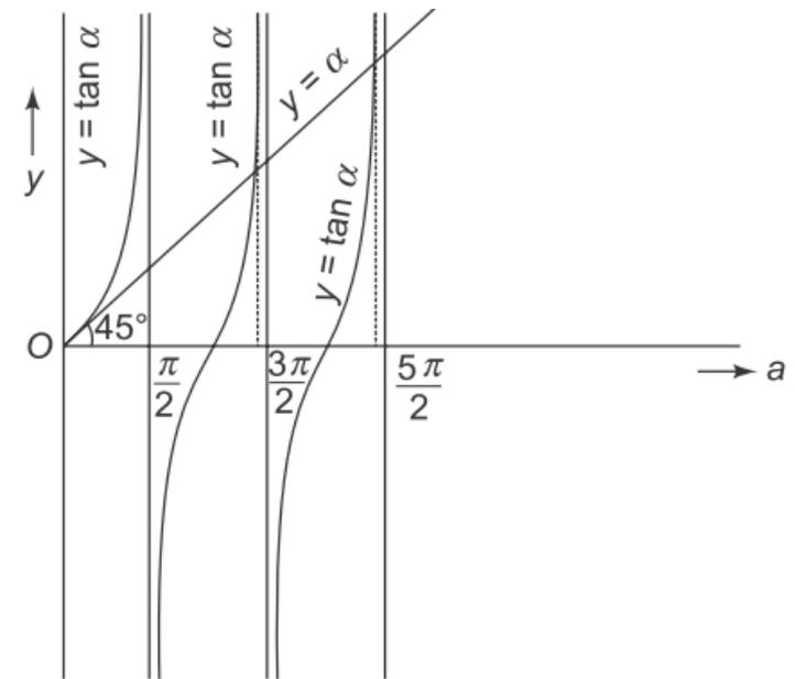
Fig. 13.5 The plot of  $y = \alpha$  and  $y = \tan \alpha$
