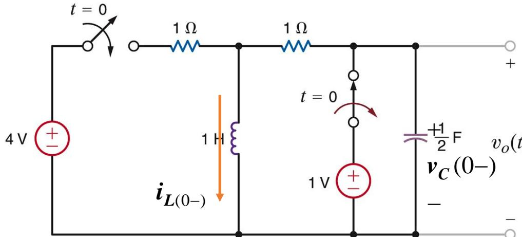
Assume steady state for  $t < 0$  and determine voltage across capacitors and currents through inductors
