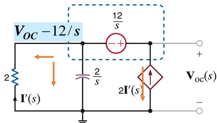
$$\frac{V_{oc} - 12/s}{2} + \frac{V_{oc} - 12/s}{2/s} - 2I' = 0$$
