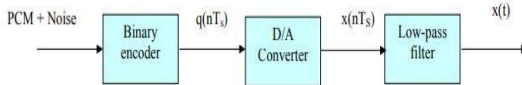
Figure.(3): PCM demodulator
