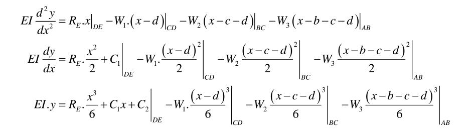
Q. A simply Supported beam carry 2 point loads 64 KN & 48 KN at B and C points. Find the deflection under each load.
