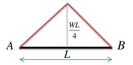
Step (3) A fixed beam is considered as a simply supported beam having fixing moments at both the ends. Since it is a case of symmetrical loading so equal fixing moments are required at both ends.
