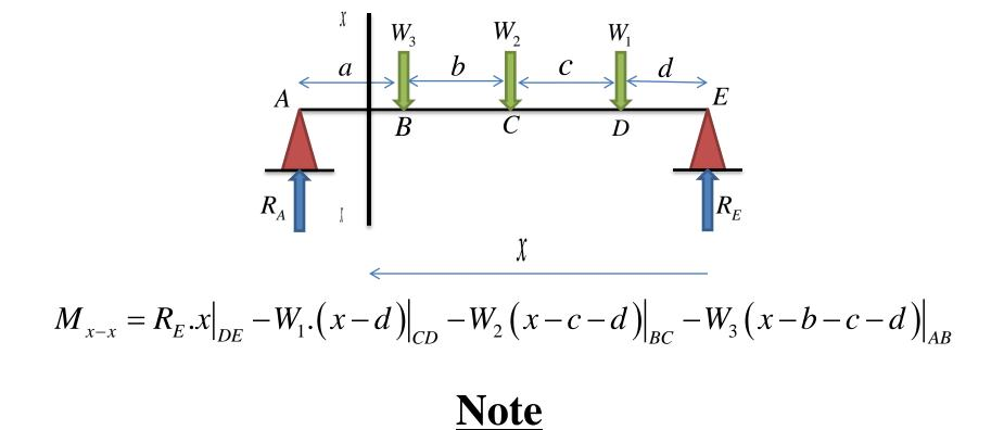
In the bending moment equation by substituting any value of x, if the form in the **bracket** become negative, delete that term completely.
