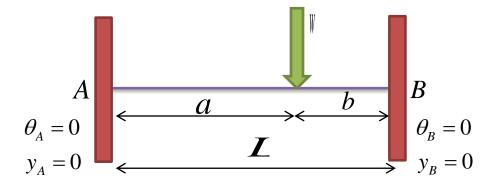
Step (1) A fixed beam is considered as a simply beam with the given loading condition.
