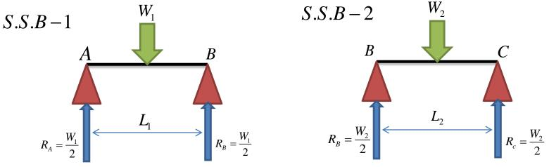
3. Draw the Bending moment diagram for SSB-1 and SSB-2
