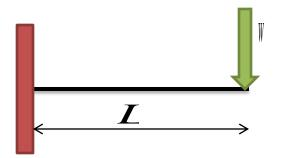
Q. For the cantilever beam as known in the figure determine the maximum slope and deflection. For section AC the flexural rigidity is 2EI and for CB section is EI.
