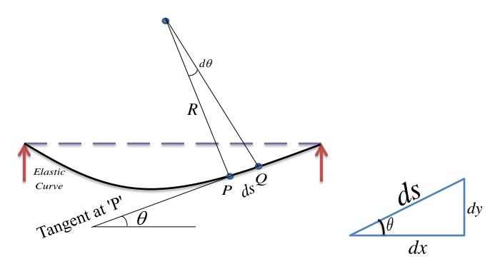
Where dx and dy represent the projected lengths of the segment ds along X and Y axes.
