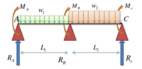
On simplification the term  $-\frac{6A_1\overline{x_1}}{L_1} - \frac{6A_2\overline{x_2}}{L_2}$  has become,  $-\frac{6A_1\overline{x_1}}{L_1} - \frac{6A_2\overline{x_2}}{L_2} = -\frac{w_1L_1^3}{4} - \frac{w_2L_2^3}{4}$
