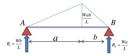
**Step (3)** A fixed beam is considered as a simply supported beam having fixing moments at both the ends. Since it is a case of unsymmetrical loading so unequal fixing moments are required at both ends.
