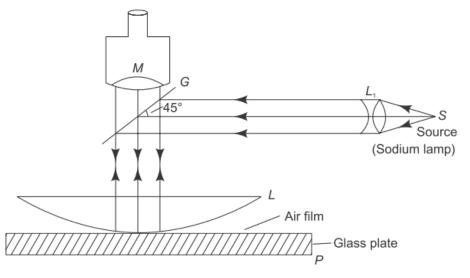
We know that for dark rings,  $D_n^2 = 4n \ \lambda R$ For (n+p) dark ring,  $D_{n+p}^2 = 4 \ (n+p) \ \lambda R$ Both will give  $D_{n+p}^2 - D_n^2 = 4p \ \lambda R$  $\lambda = \frac{D_{n+p}^2 - D_n^2}{4pR}$
