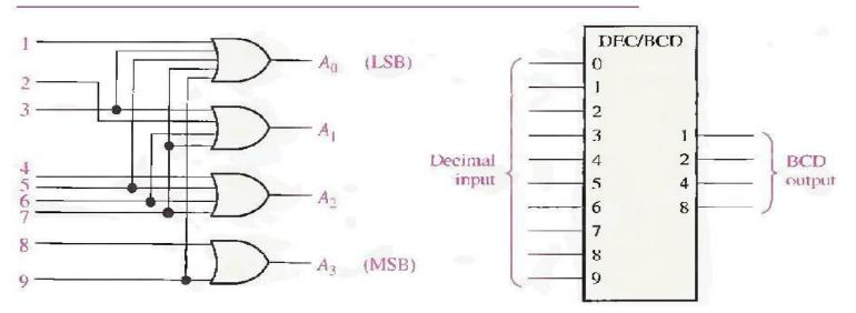
Fig : Logic circuit and symbol for 10-4 encoder
