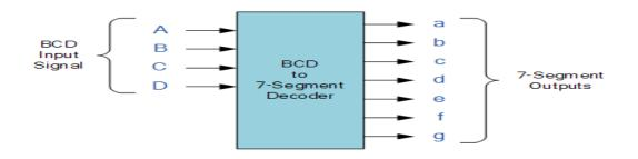
Fig: logical symbol of BCD-7 segment decoder
