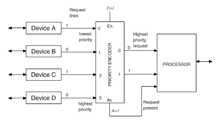
Figure 9.17: Resolving interrupt requests using a priority encoder.
