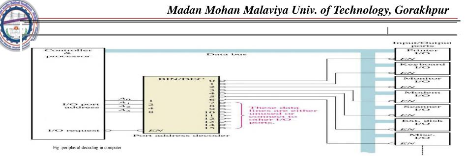
•Computer must communicate with a variety of external devices called peripherals by sending and/or receiving data through what is known as input/output (I/O) ports
