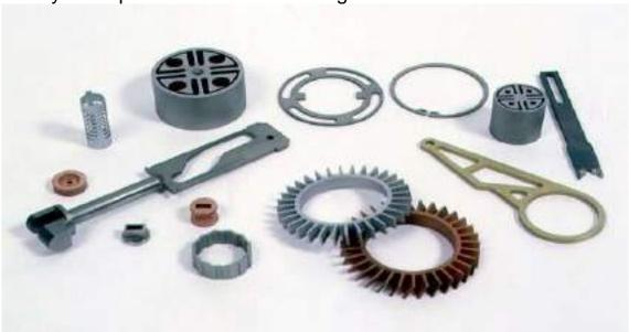
Figure 14: Difficult internal parts made by EDM process
