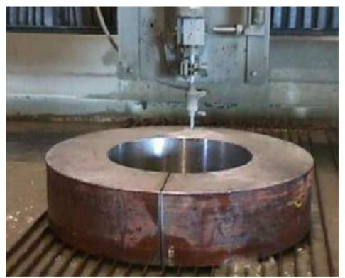
Figure 5: Abrasive water jet cutting
