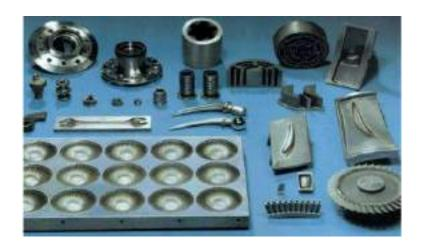
Figure 9: Parts made by ECM
