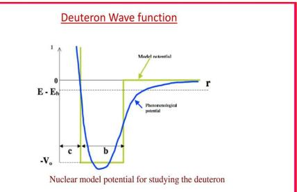
To simplify the analysis of the deuteron, we assume that the nucleonnucleon potential is *a three-dimensional square well*, as shown in the figure *a*:
