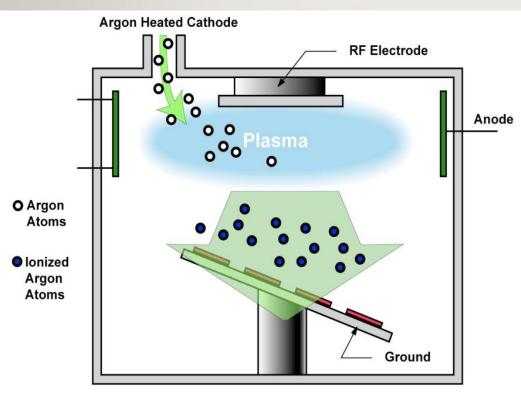
Ion Beam Milling
