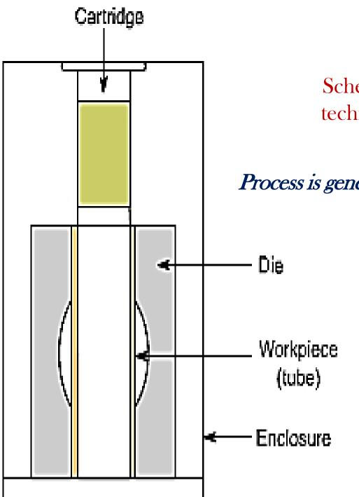
Schematic illustration of contact technique of explosive forming.
