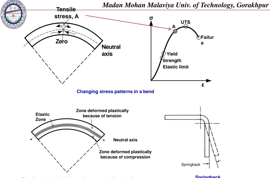
Elastic and plastic deformation zones during bending
