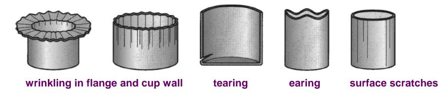
**Wrinkling** in flange and cup wall: This is like ups and downs or waviness that is developed on the flange. If the flange is drawn into the die hole, it will be retained in cup wall region.
