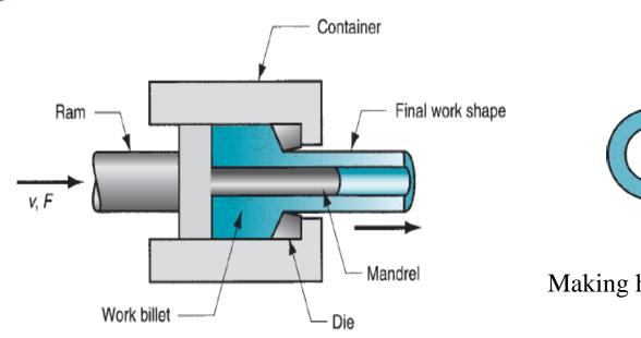
Making hollow shapes using direct extrusion
