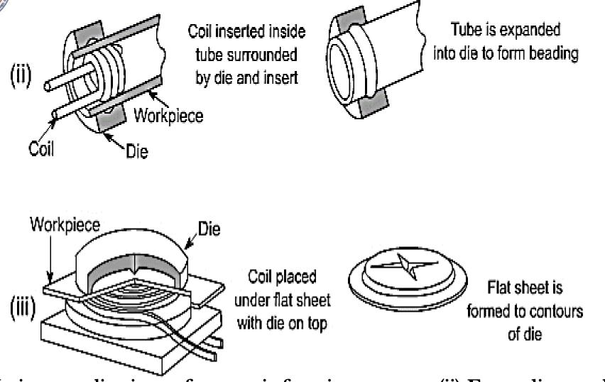
Various applications of magnetic forming process. (ii) Expanding, and (iii) Embossing or blanking.
