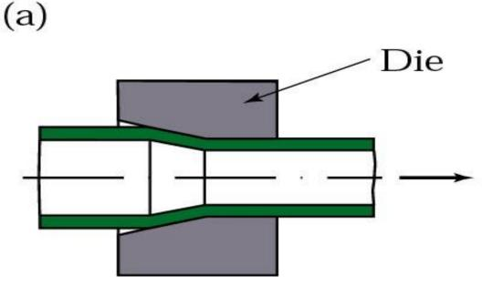
The tube, while passing through the die, shrinks in outer radius from the original radius
