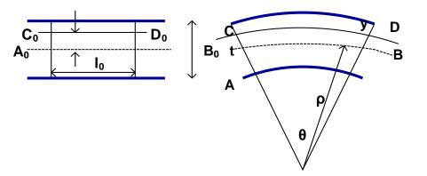
For our analysis, it may be assumed that a plane normal section in the sheet will remain plane and normal and converge on the center of curvature as shown in Figure. The line  $A_0B_0$  at the middle surface may change its length to AB, if the sheet is under stretching during bending. The original length  $I_o$  becomes,  $I_s = \rho \theta$ . A line  $C_0D_0$  at a distance y from the middle surface will deform to a length,
