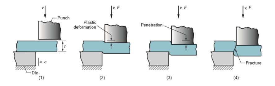
• FIGURE 1. Shearing of sheet metal between two cutting edges: (1) just before the punch contacts work; (2) punch begins to push into work, causing plastic deformation; (3) punch compresses and penetrates into work causing a smooth cut surface; and (4) fracture is initiated at the opposing cutting edges that separate the sheet.
