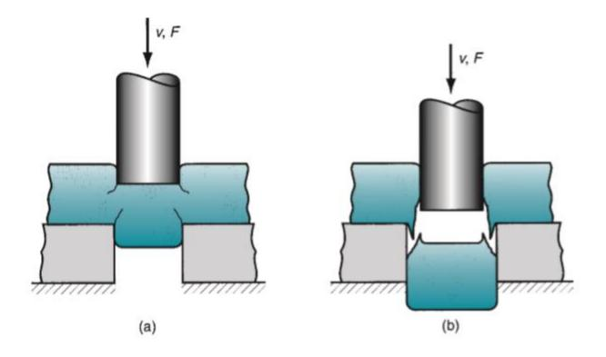
• Effect of clearance: (a) clearance too small causes less-than optimal fracture and excessive forces; and (b) clearance too large causes oversized burr.
