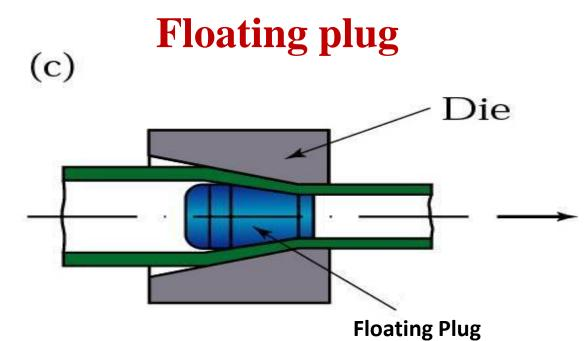
•A tapered plug is placed inside the tube.
