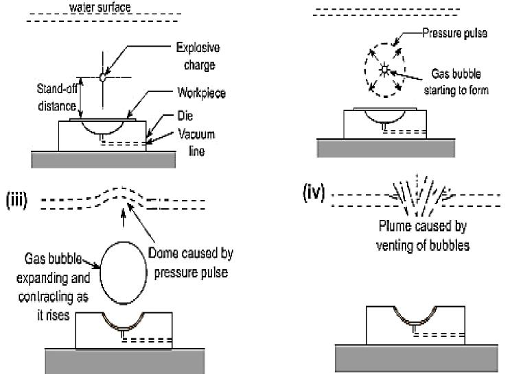
Sequeuce of underwater explosive forming operations.(i) explosive charge is set in position (ii) pressure pulse and gas bubble are formed as the detonation of charge occurs, (iii) workpiece is deformed, and (iv) gas bubbles vent at the surface of water.
