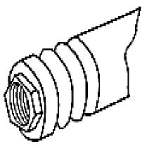
Coil around tube is compressed into grooves of fitting
