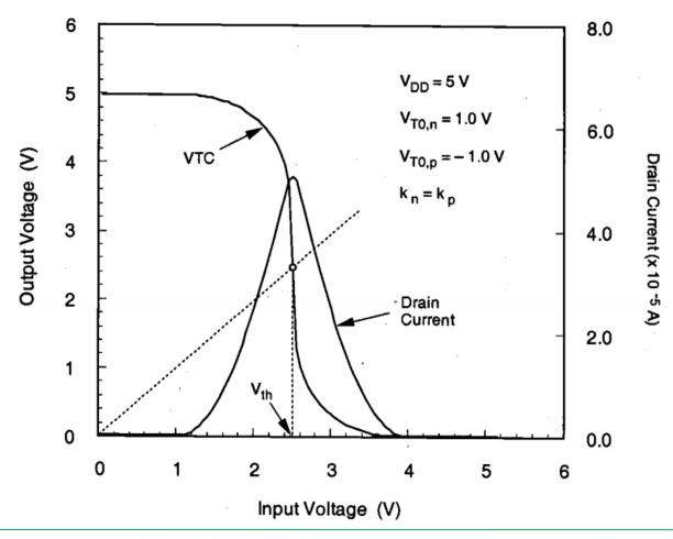
**Fig.** Typical VTC and the power supply current of a CMOS inverter circuit.
