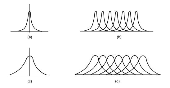
Effect of cross-sectional intensity on resolution (a) Spot with well defined edges (b) Several such overlapping spots (c) Wider spot with less height (d) Several wider overlapping spots
