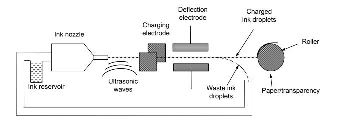
Schematic of continuous flow inkjet printer
