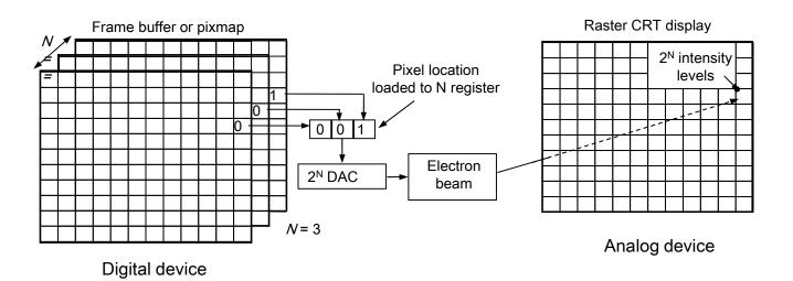
N-bit-plane Monochrome gray level frame buffer raster CRT display
