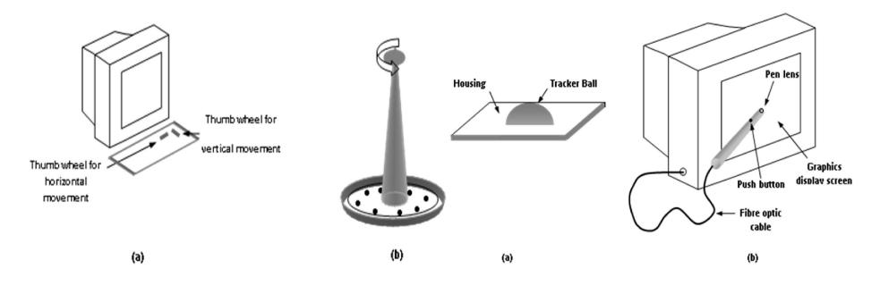
**Cursor Control Input Devices** (a) Thumbwheels (b) Joystick Cursor Control Input Devices (a) Tracker ball (b) Light Pen
