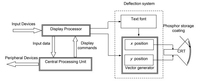
DVST Display System (Display file is missing)
