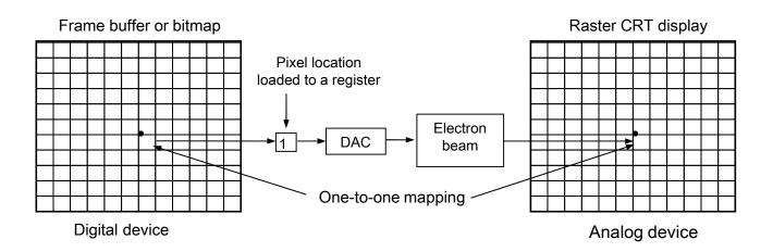
Single-bit-plane monochrome frame buffer raster CRT display
