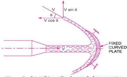
Fig. 3 Jet striking a fixed curved plate at centre.
