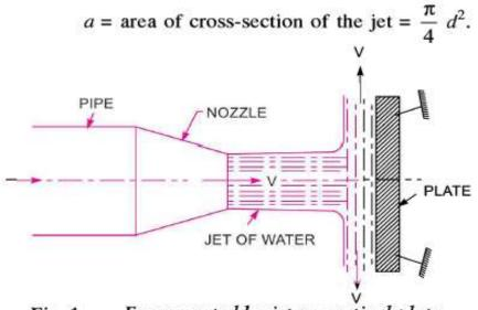
Fig. 1 Force exerted by jet on vertical plate.
