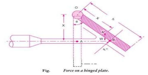
x = distance of the centre of jet from hinge O,  $\theta =$  angle of swing about hinge,
