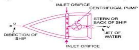
Fig. Inlet orifices are at right angles.
