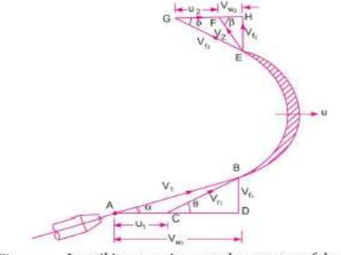
Fig. Jet striking a moving curved vane at one of the tips.
