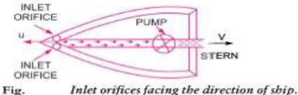
as in this case the water enters with a velocity equal to the velocity of the ship, *i.e.*, with a velocity u.
