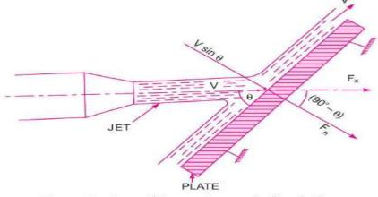
Fig. 2 Jet striking stationary inclined plate.
