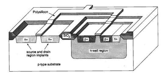
**Fig.** Using a set of two masks, the n+ and p+ regions are implanted into the substrate and into the n-well, respectively. Also, the ohmic contacts to the substrate and to the n-well are implanted in this process step.
