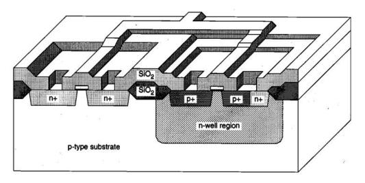
Fig. An insulating silicon dioxide layer is deposited over the entire wafer using CVD. Then, the contacts are defined and etched away to expose the silicon or polysilicon contact windows. These contact windows are necessary to complete the circuit interconnections using the metal layer, which is patterned in the next step.
