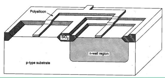
Fig. The polysilicon layer is deposited using chemical vapor deposition (CVD) and patterned by dry (plasma) etching. The created polysilicon lines will function as the gate electrodes of the nMOS and the pMOS transistors and their interconnects.
