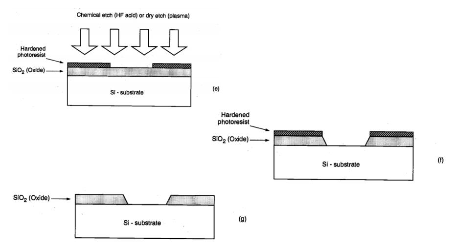
Fig. Process steps required for patterning of silicon dioxide (continued).
