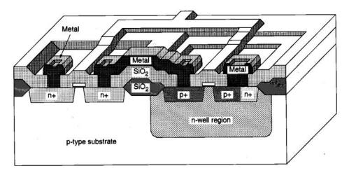
Fig. Metal (aluminum) is deposited over the entire chip surface using metal evaporation, and the metal lines are patterned through etching. Since the wafer surface is non-planar, the quality and the integrity of the metal lines created in this step are very critical and are ultimately essential for circuit reliability.
