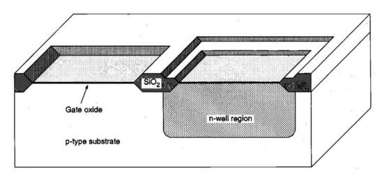
Fig. The creation of the n-well region, a thick field oxide is grown in the areas surrounding the transistor's active regions, and a thin gate oxide is grown on top of the active regions. The thickness and the quality of the gate oxide are two of the most critical fabrication parameters, since they strongly affect the operational characteristics of the MOS transistor, as well as its long-term reliability.
