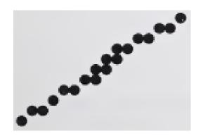
Uneven line density caused by bunching of dots.
