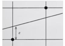
the y coordinate of the current point. A positive e value indicates that the exact path of the line lies above the current point; therefore the y coordinate is incremented, and 1 is subtracted from e. If e is negative the y coordinate value is left unchanged.
