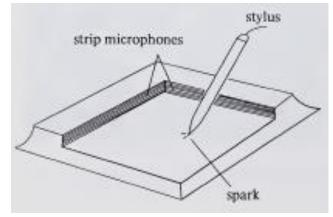
The stylus has a small piece of ceramic mounted close to its tip, and at regular intervals a small spark is generated across the surface of the ceramic between two electrodes. The microphones pick up the pulse of sound generated by the spark, and two counters record the delay between creating the spark and receiving the sound. These two delays are proportional to the stylus distance from the two edges of the tablet where the microphones are mounted. They can therefore be used as x and y values.
