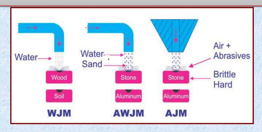
HOW DOES IT WORK? K.E. of WATER AND / OR ABRASIVE PARTICLES MAKES IT TO HAPPEN.
