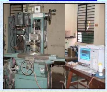
DIGITAL PHOTOGRAPH OF FLEXIBLE MAGNETIC ABRASIVE BRUSH (FMAB)
