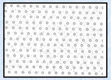
HOLE  $\phi$  =0.006 mm (6  $\mu$ m) HOLES DENSITY = 200,000 / cm<sup>2</sup> THICKNESS = 0.12 mm TIME= 2 $\mu$ s / HOLE
