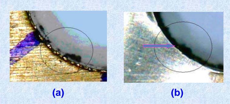
Drilled hole edge (a) before, (b) after deburring
