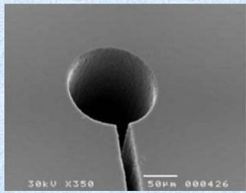
MICRO FLUIDIC DEVICE IN SILICON SHOWING LASER DRILLED VIA HOLE AND CONNECTING CHANNEL
