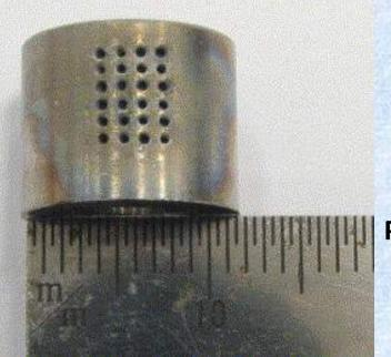
MICRO-HOLES PRODUCED ON A  $Ti_6AI_4V$  CYLINDER USING JET-EMM
