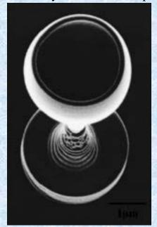
Micro wine glass with 2.75 μm external diameter and 12 μm height.
