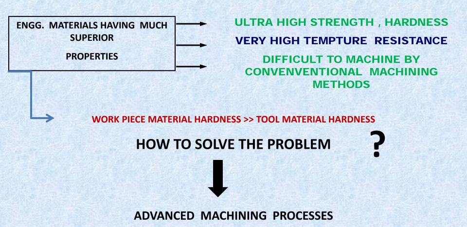
WORKPIECE HARDNESS DOES NOT MATTER IN AMPS
