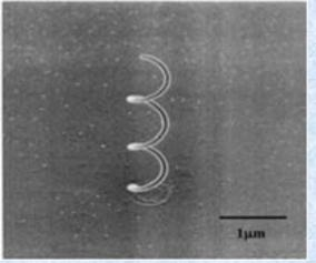
Coil 700 nm pitch, 80 nm line width, diamond like amorphous carbon, Fabricated by FIB induced deposition
