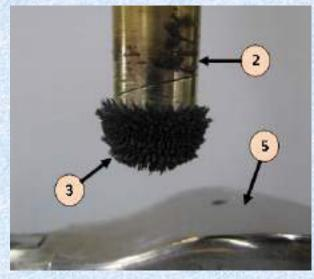
(1- CNC milling M/c head, 2- MR finishing tool, 3- MR polishing fluid, 4- fixture for knee joint implant (Ti6Al4V), 5- knee joint implant)
