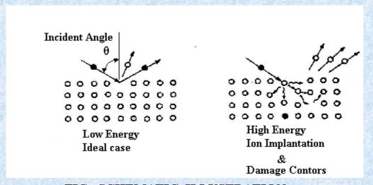
FIG. SCHEMATIC ILLUSTRATION
