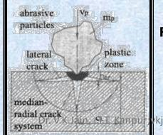
FORCES ACTING ON EACH PARTICLE AND PARTICLE SIZE WILL DEC IDE THE SCALE OF MATERIAL REMOVED: MACRO, MICRO, NANO
