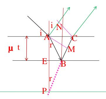
Path diffidence between interfering waves can be given as  $(AB+BC) \mu$ -AN  $=(AB+BC) \mu$ - $\mu$ MC  $=(AB+BM) \mu$  $=(PB+BM) \mu$  $= \mu$ PM  $= 2 \mu t \cos r$ Now the actual path diff.  $2 \mu t \cos r \pm \lambda/2$
