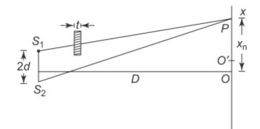
In the absence of plate (t = 0), the distance of nth bright fringe from centre O is  $\frac{D}{2d}$  n $\lambda$ . Therefore, the displacement of nth bright fringe is given by
