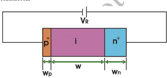
The most common semiconductor photo detector is the PIN photodiode.
