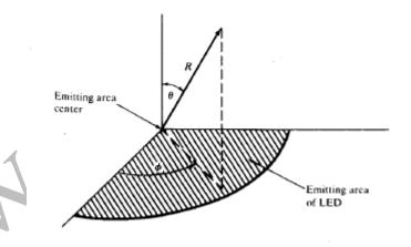
Here the figure shows a spherical coordinate system characterized by R,  $\theta$  and  $\phi$  with the polar axis. The radiance may be a function of both  $\theta$  and  $\phi$  and can also vary from point to point on the emitting surface.
