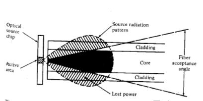
Here, the fiber end face is centered over emitting surface of the source and is positioned as close as possible. So, the power coupled is:
