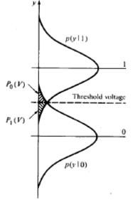
RECEIVER SENSITIVITY: Optical communication system use a BER value to specify the performance requirement for a
