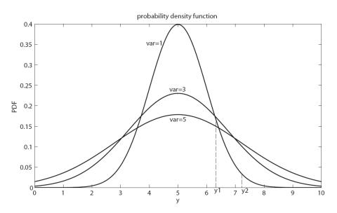
Figure 1.1 Gaussian PDF for mean 'm=5'
