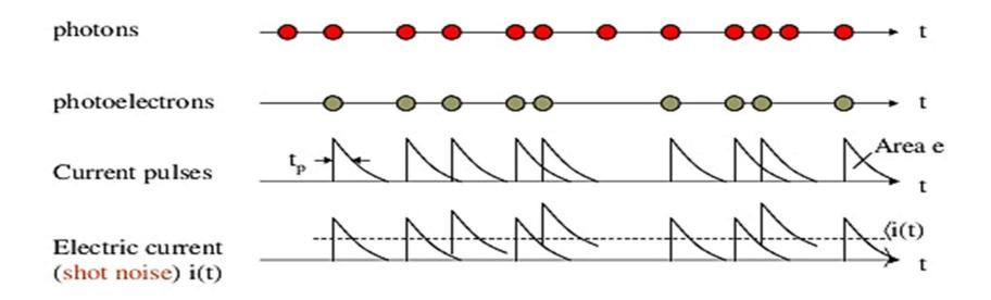
The photocurrent induced in a photodetector circuit comprises a superposition of current pulses, each associated with a detected photon. The individual pulses illustrated are exponentially decaying step functions but they can assume an arbitrary shape.
