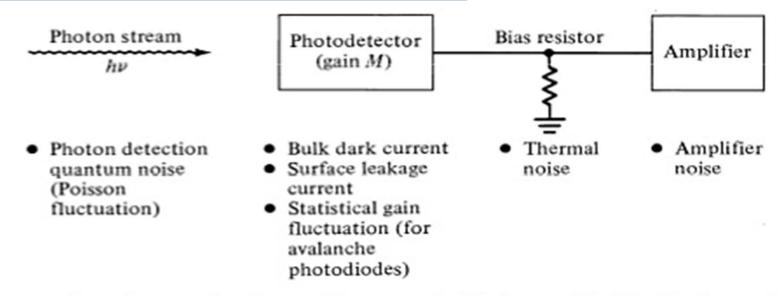
Photon noise – the most fundamental source of noise is associated with the random arrivals of the photons (usually described by Poisson statistics)
