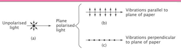
Fig. 14.5 (a) Unpolarised light and (b, c) linearly polarised light
