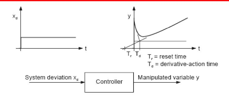
✓ This is one of the most powerful but complex controller mode operations combines the proportional, integral and derivative modes. The output for this mode can be expressed as:
