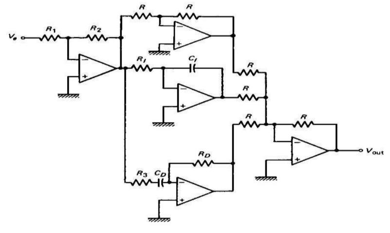
$$-Vout = (\frac{R_2}{R_1})Ve + (\frac{R_2}{R_1})\frac{1}{R_1C_I}\int V_e dt + (\frac{R_2}{R_1})R_DC_D\frac{dV_e}{dt} + Vout(0)$$
