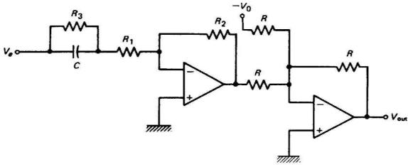
$$Vout = (\frac{R_2}{R_1 + R_3})Ve + (\frac{R_2}{R_1 + R_3})R_3C\frac{dVe}{dt} + Vo$$
