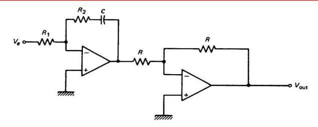
$$Vout = (\frac{R_2}{R_1})Ve + (\frac{R_2}{R_1})\frac{1}{R_2C}\int_{0}^{t} V_e dt + Vout(0)$$
