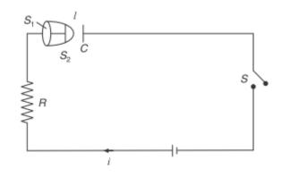
Let us consider a plane surface  $S_1$  and a hemispherical surface  $S_2$  around the condenser plate as shown in Fig. 17.1. Let both surfaces be bounded by the same closed path I, and applying Ampere's law to the surface  $S_1$ , we get
