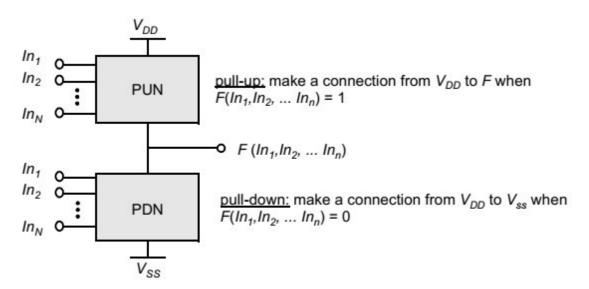
Complementary logic gate as a combination of a PUN (pull-up network) and a PDN (pull-down network)
