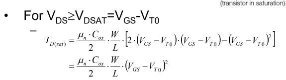
The drain current becomes a function only of V<sub>GS</sub>, beyond the saturation boundary
