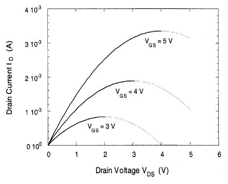
The drain current-drain voltage curves shown on page 104 reach their peak value for  $V_{DS} = V_{GS} - V_{T0}$ . Beyond this maximum, each curve exhibits a *negative* differential conductance, which is not observed in actual MOSFET current-voltage measurements (section shown by the dashed lines). We must remember now that the drain current equation (3.32) has been derived under the following voltage assumptions,
