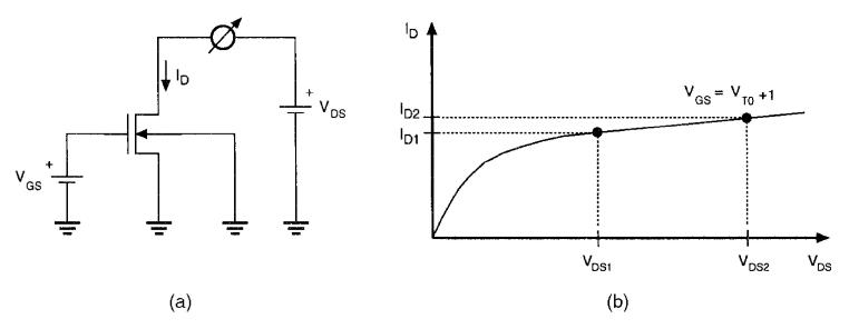
(a) Test circuit arrangement and (b) measured data for experimental Figure 3.23 determination of the channel length modulation coefficient  $\lambda$ .
