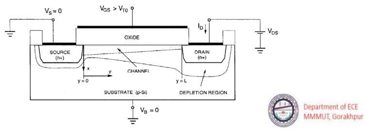
Figure 3.15 Cross-sectional view of an n-channel transistor, operating in linear region.
