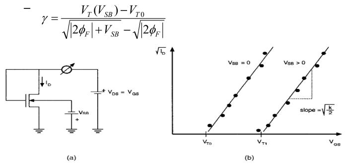
**Figure 3.22** (a) Test circuit arrangement and (b) measured data for experimental determination of the parameters  $k_{D}$ ,  $V_{T0}$ , and  $\gamma$ .
