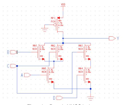
Fig. using Pseudo NMOS logic
