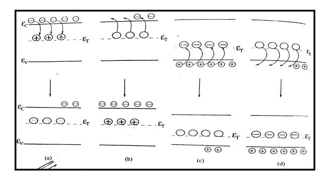
Illustration of (a) electron capture, (b) electron emission, (c) hole capture, and (d) hole emission. The deep levels in (a) and (b) are electron traps and those in (c) and (d) are hole traps
